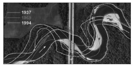
FIGURE 2 Channel migration can have wide-ranging effects on bridge abutments that rest on floodplain soils. Aboe, Wapsipinicon River near DeWitt, Iowa.
