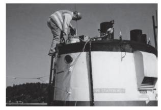
Washington State Ferries crew member performs emissions testing on the *MIV Rhododendron*. The entire fleet has switched to cleaner diesel or biodiesel fuels to reduce sulfur dioxide emissions.
