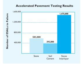
FIGURE I Performance of stone interlayer compared with soil-cement and crushed rock.
