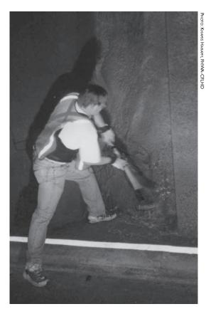
Investigator uses a title hammer to survey seismic characteristics of Zion–Mt. Carmel Tunnel.
