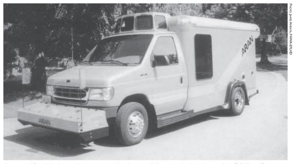
Automated Road Analyzer vehicle is equipped with state-of-the-art technology that enables FHVVA staff to collect pavement data on the roadway network within the National Park System.
