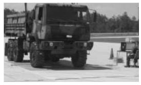
Demonstration of weigh-in-motion (WIM) at Fort Bragg, North Carolina, May 2003, with truck moving over portable system.
