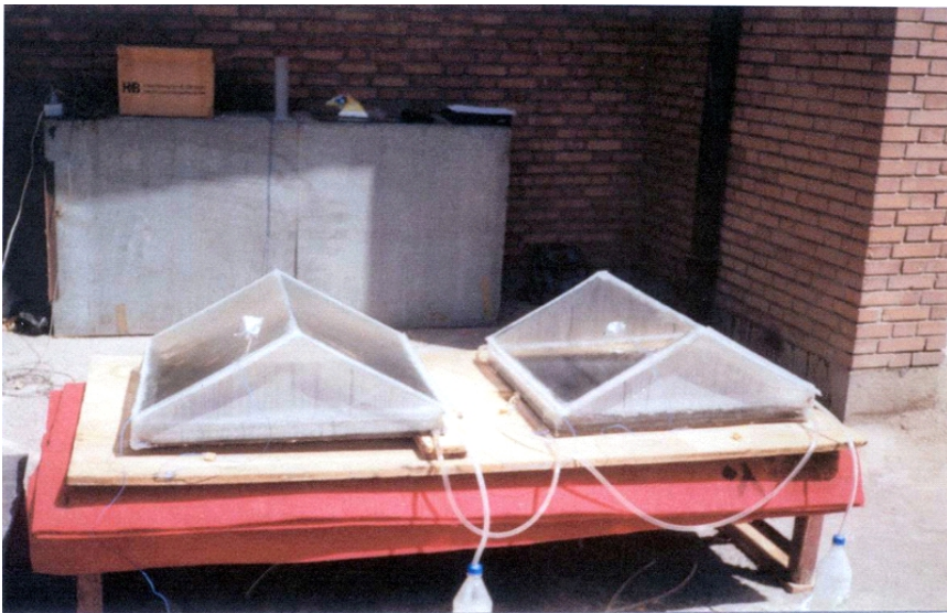
FIGURE 5 The experiment setup of solar stills built of Plexiglass.
