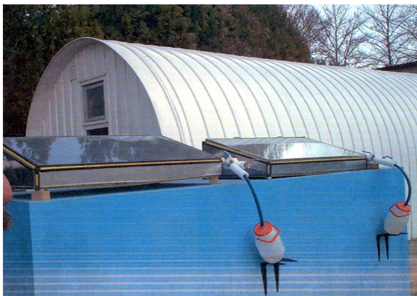
FIGURE 4 The experiment setup of solar stills built of stainless steel.
