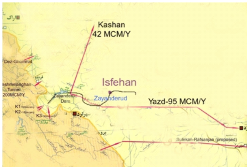
FIGURE 5 Interbasin transfers from Persian Gulf Basins to Central Basin.
