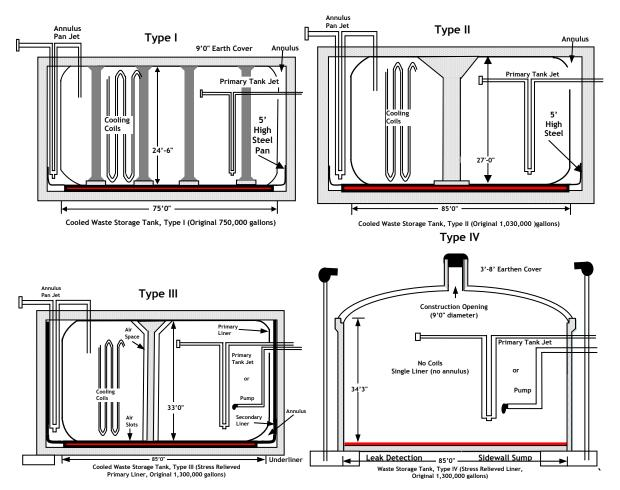
FIGURE 1 Diagrams of tank types at the Savannah River Site (not drawn to scale). There are twelve Type I tanks, four Type II tanks, twenty-seven Type III (and IIIA) tanks, and eight Type IV tanks in the tank farms. Risers are not depicted in most of these diagrams but are present on each tank.
