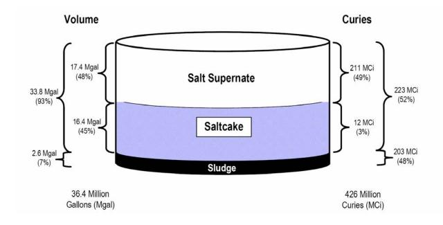
FIGURE 2 Aggregated volume and radioactivity distributions among the tank waste phases in all tanks at the Savannah River Site as of December 2004. SOURCE: DOE (2005a).
