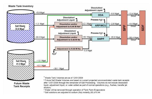
FIGURE 8 Volume flows in DOE's salt waste processing plans. NOTES: 1 Mgal = approximately 3,800 m<sup>3</sup>. DDA = Deliquification, Dissolution, and Adjustment; ARP = Actinide Removal Process; MCU = Modular Caustic-Side Solvent Extraction Unit; SWPF = Salt Waste Processing Facility; SPF = Saltstone Production Facility; SDF = Saltstone Disposal Facility. SOURCE: Adapted from DOE (2005a)
