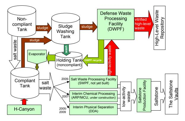
FIGURE S-2 Waste flows in the Savannah River Site waste management plans. Note that the sizes do not necessarily scale with the sizes of the waste flows.
