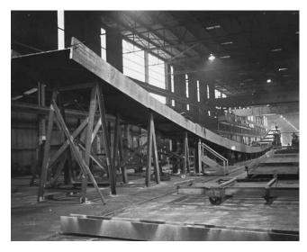
FIGURE 6 Progressive girder assembly.
