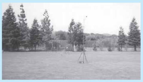
Microphones and sensors measuring traffic noise.
