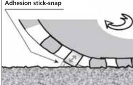
FIGURE 4 (*at left*) Slipstick motion of the tread block on pavement (2).
