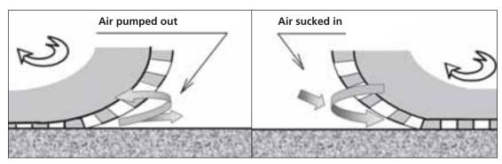
FIGURE 3 Air pumping at (left) entrance and (right) exit of the contact patch (2).
