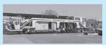
BART railgrinder used to reduce noise levels.
