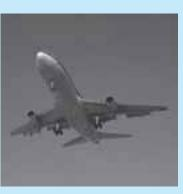
Lowered landing gear contributes to airframe noise in flight.
