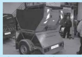
Trailer used in the Netherlands for sound measurement by the close-proximity method.
