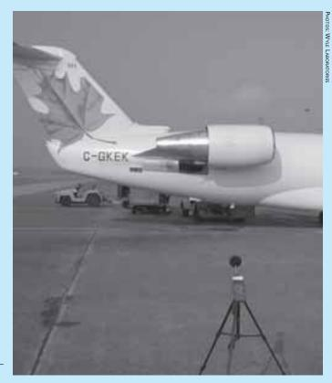
sources. The first is called compressor whine, the high-pitched whistling from the front of the engine. The spinning machinery inside the engine is the cause, most noticeably when an aircraft is approaching a runway. Sound-absorbing liners along the inlet of the jet engine can reduce compressor whine.
