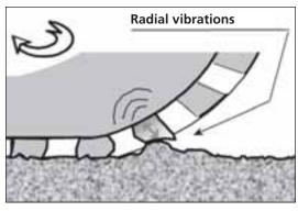
FIGURE 2 Vibration caused by tread block-pavement impact (2).
