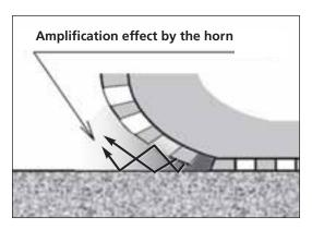
FIGURE 6 Horn effect or amplification created by the tire and pavement (2).
