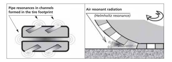
FIGURE 7 Sound amplification caused (*left*) by organ pipe resonances in channels in the tire footprint, and (*right*) by Helmholtz resonator geometries within the contact patch (2).
