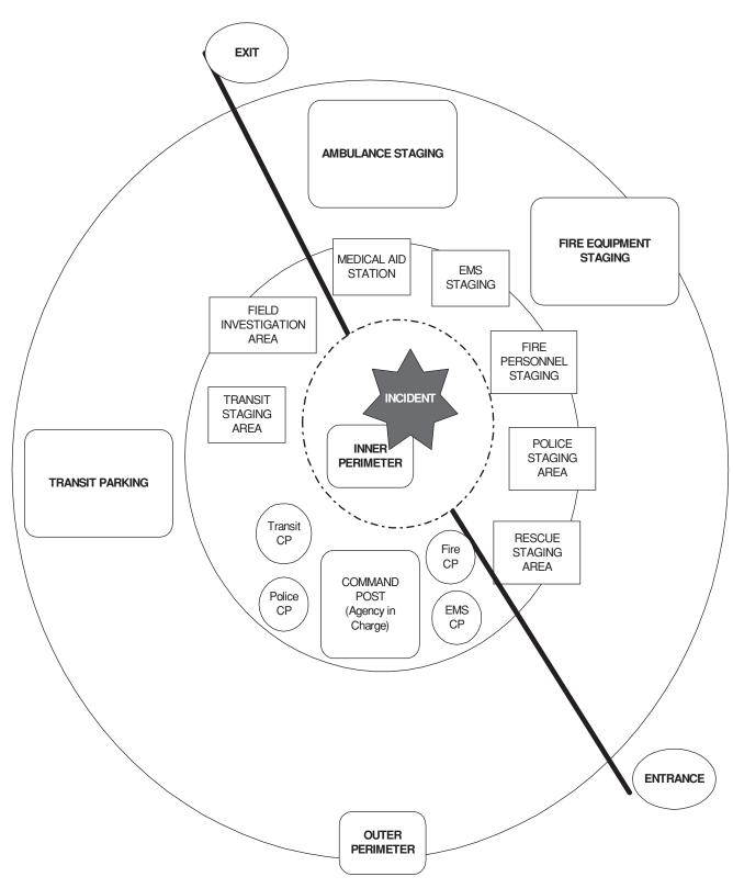
Figure 7-6. Schematic for response in transportation environment.
