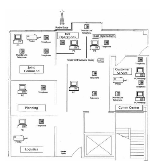
Figure 3-4. Sample joint command emergency operations center.
