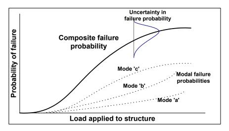
FIGURE 3-2 Form of result of structural reliability analysis of shore protection structure.
