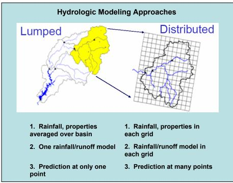
FIGURE 3-3 Differences between lumped and distributed model approaches. SOURCE: Adapted from Smith et al., 2004a.
