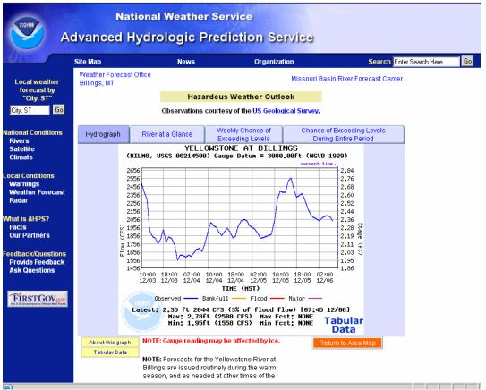
FIGURE 2-5 Example of how AHPS hydrograph information is linked to USGS gage data. SOURCE: http://ahps2.wrh.noaa.gov/ahps2/hydrograph.php?wfo=byz&gage=bilm8&view=1,1,1,1,1,1.
