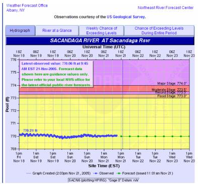
FIGURE 4-1 Hydrograph and forecast plot (Northeast RFC). SOURCE: http://newweb.erh.noaa.gov/ahps2/hydrograph.php?wfo=aly&gage=sacn6&view=1,1,1,1,1,1,1.
