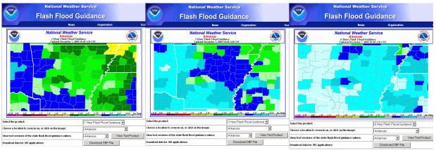
FIGURE 4-6 From left to right, flash-flood guidance for 1-hour, 3-hour, and 6-hour durations for Arkansas.
