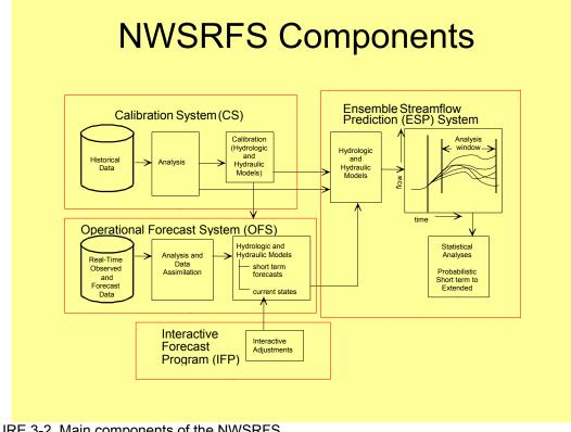
FIGURE 3-2 Main components of the NWSRFS. SOURCE: Adapted from McEnery et al., 2005.
