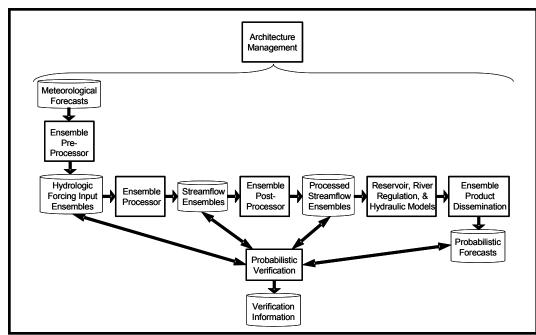
FIGURE 3-4 System components for the ESP. SOURCE: NWS, 2004.
