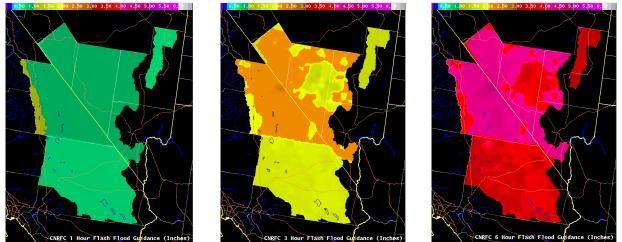
FIGURE 4-7 From left to right, AHPS products for flash-flood guidance for 1-hour, 3-hour, and 6-hour durations (California Nevada RFC, Sacramento, CA). SOURCE: http://www.wrh.noaa.gov/cnrfc/flashFloodGuidance.php.
