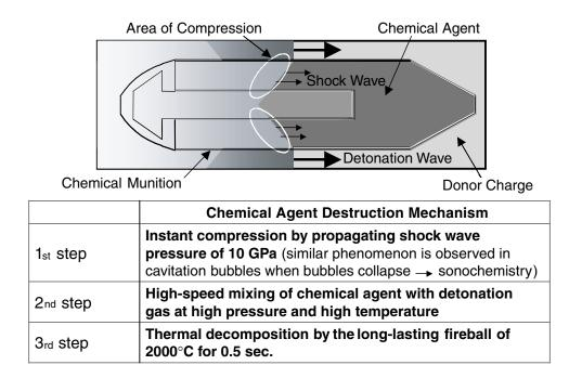
FIGURE 4-2 DAVINCH three-stage destruction mechanism. SOURCE: Joseph Asahina, Kobe Steel, December 8, 2005.
