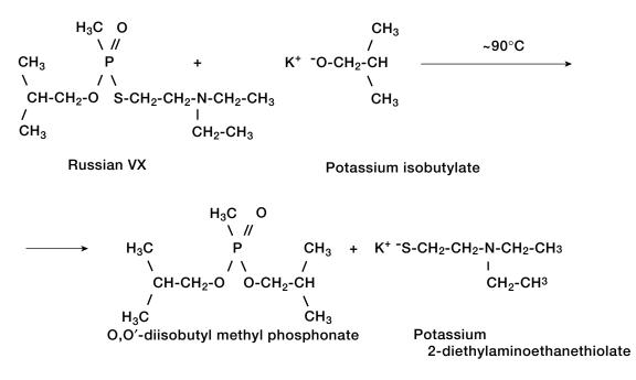
FIGURE 5-1 Reaction of Russian VX and potassium isobutylate. SOURCE: Bechtel, 1996.
