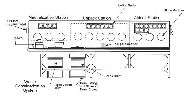
FIGURE 1-2 Diagram of RRS operations trailer. SOURCE: U.S. Army, 2001a.
