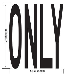
FIGURE 3B-20 Example of Elongated Letters for Word Pavement Markings
