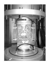
Figure 10. Confined test set-up.
