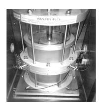
*Figure 11. Test set-up within triaxial cell with mounted radial LVDTs.*
