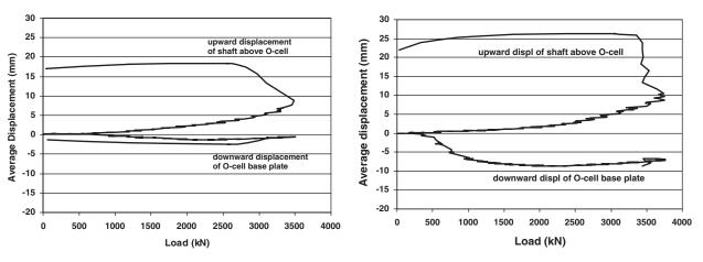
FIGURE 63 Results of single O-cell load tests: (left) Shaft No. 1; (right) Shaft No. 3 (Gunnink and Kiehne 2002).
