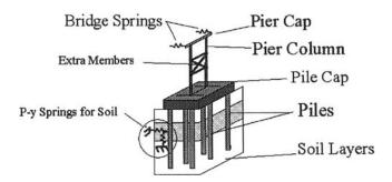
FIGURE 44 Florida pier model for structure and foundation elements (Hoit et al. 1997).
