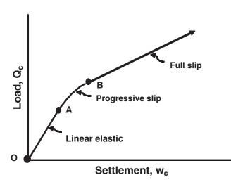
FIGURE 19 Idealized load-displacement behavior.
