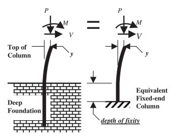
FIGURE 47 Depth of fixity for equivalent fixed-end column.
