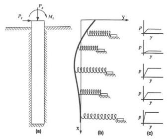
FIGURE 36 Subgrade reaction model based on *p*-*y* curves (Reese 1997).
