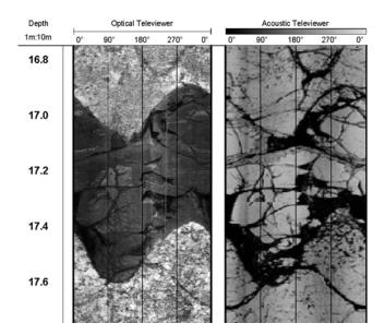
FIGURE 9 Optical and acoustic televiewer images of a 50-cm diorite dike in granite (Eliassen et al. 2005).
