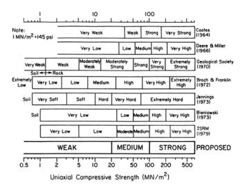
FIGURE 18 Classification for unweathered rock material strength (Kulhawy et al. 1991).
