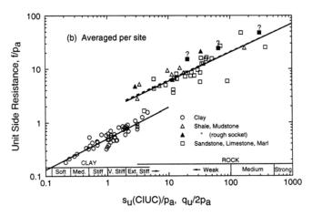
FIGURE 24 Unit side resistance versus strength (Kulhawy and Phoon 1993).
