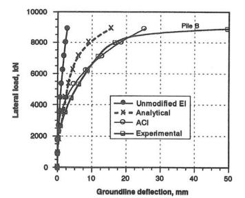
FIGURE 39 Measured and analytical deflection curves, socket in sandstone (Reese 1997).
