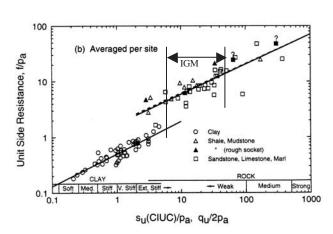
FIGURE 17 Side resistance versus geomaterial strength (Kulhawy and Phoon 1993).
