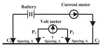
FIGURE 7 Field configuration for resistivity test.
