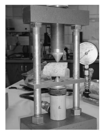
FIGURE 13 Point load test setup.
