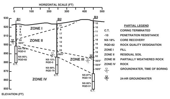
FIGURE 81 Typical Piedmont subsurface profile (after Schwartz 1987).
