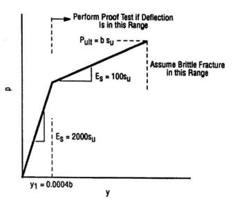
FIGURE 40 Recommended *p*-*y* curve for strong rock (Ensoft, Inc. 2004).
