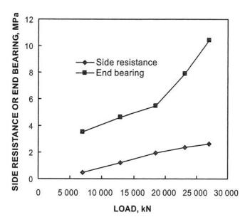
FIGURE 60 Unit side and base resistance versus axial load (Zhan and Yin 2000).
