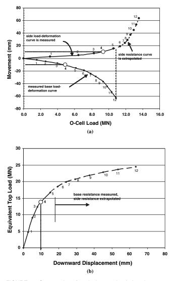
FIGURE 65 Construction of equivalent top-loaded settlement curve from O-cell test results (*a*) O-cell measured loaddisplacement; (*b*) equivalent top-load settlement results.
