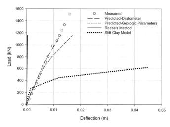
FIGURE 42 Measured lateral load deflection versus predicted (Gabr et al. 2002).
