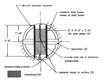
FIGURE 73 Top view of O-cell arrangement for lateral split socket test (O'Neill 1997).
