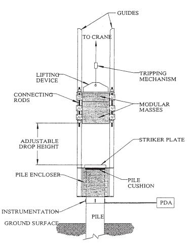
FIGURE 69 Schematic of drop weight system (Paikowsky et al. 2004c).
