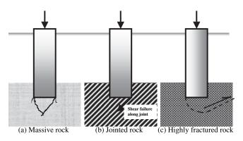
FIGURE 14 Base failure modes illustrating different operational shear strength conditions.
