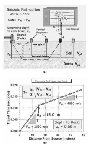
FIGURE 5 Seismic refraction method (Mayne et al. 2001): (*a*) field setup and procedures; (*b*) data reduction for depth to hard layer.
