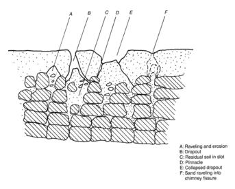
FIGURE 79 Features of karstic terrain (Knott et al. 1993).
