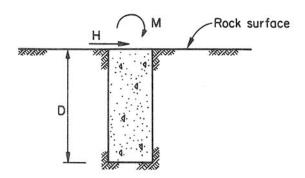
FIGURE 45 Lateral loading of rock-socketed shaft (Carter and Kulhawy 1992).
