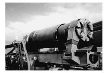
FIGURE 55 Downhole hammer tool for drilling in hard rock.
