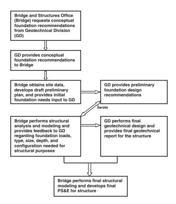
FIGURE 2 Design process for Load and Resistance Factor Design (Washington State DOT 2005). PS&E = <u>P</u>lans, <u>Specifications</u>, & <u>E</u>stimates.
