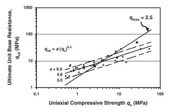
FIGURE 33 Unit base resistance versus intact rock strength (derived from Zhang and Einstein 1998).
