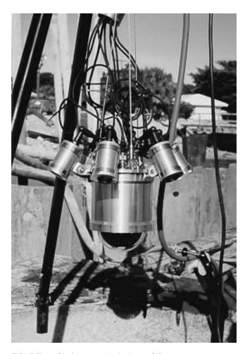
FIGURE 78 Shaft inspection device or SID.
