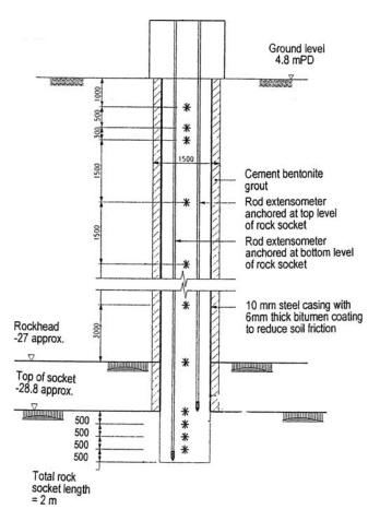
FIGURE 59 Details of instrumented rock-socketed shaft (Zhan and Yin 2000).
