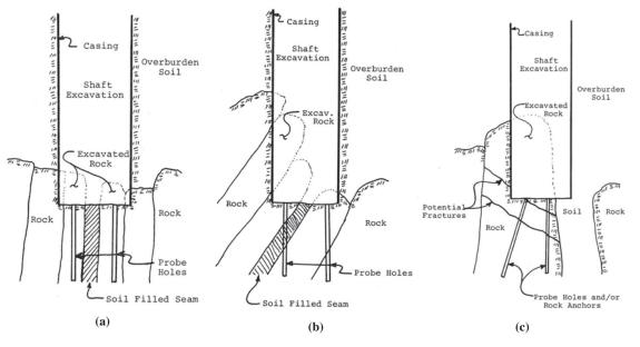
FIGURE 80 Commonly encountered conditions for shafts in pinnacled limestone (Brown 1990).
