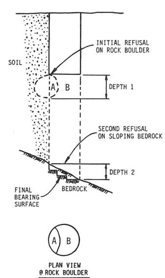
FIGURE 82 Typical drilling in Piedmont soils and rock (Schwartz 1987).
