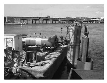
FIGURE 74 Lateral STN load test (Courtesy: L. Fontaine).
