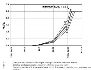
D. Fine-grained polyminerallic igneous crystalline rocks: andesite, dolerite, diabase, and rhyolite.
