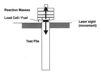
FIGURE 68 Schematic of STN load test (O'Neill et al. 1997).
