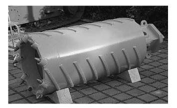
FIGURE 53 Typical single wall core barrel.
