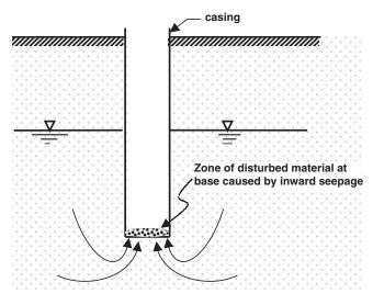
FIGURE 76 Development of disturbed base caused by high seepage gradient toward bottom of a cased hole.
