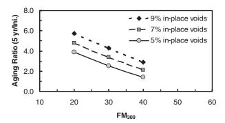
Figure 19. Predicted Mixture Age-Hardening Ratio at 25 °C and 10 Hz as a Function of In-Place Air Void Content and FM<sub>300</sub> for a MAAT of 15.6 °C.
