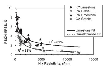
Figure 3. RSCH Permanent Shear Strain as a Function of Gyrations × Resistivity.
