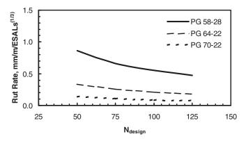
Figure 8. Effect of Binder Grade and N<sub>design</sub> on Rut Resistance of Superpave Mixtures (Design Air Voids = 4%, In-Place Air Voids = 7%).
