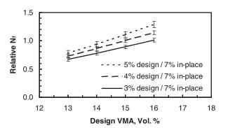
Figure 12. Effect of Design Air Voids and Design VMA on Relative In-Situ Fatigue Life, In-Place Air Voids Constant at 7% (Errors Bars = 2s Confidence Limits).
