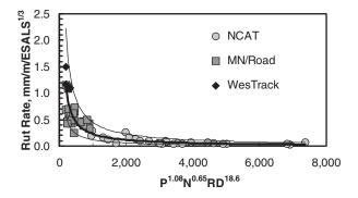
Figure 4. Relationship Between Field Rutting Rate and Proposed Function of Resistivity, N<sub>design</sub> and Air Voids; the Heavy Center Line Represents the Rutting Rate Predicted Using Equation 2 While the Thinner Lines Represent 90% Prediction Limits for New Observations.
