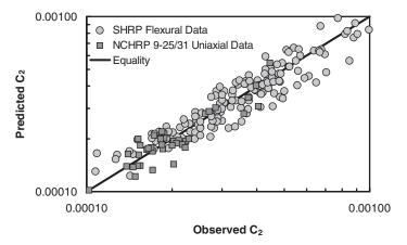
Figure 10. Predicted and Observed Values for Continuum Damage Fatigue Constant C<sub>2</sub> for SHRP Flexural Fatigue Data and NCHRP Uniaxial Fatigue Data.
