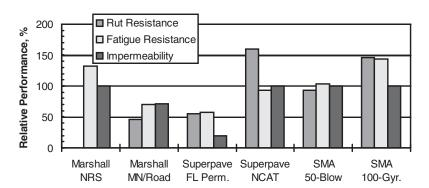
*Figure 22. Relative Performance of Various HMA Mixes Based on Volumetric Composition and Compaction; Differences in Binder Properties Ignored.*
