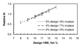
Figure 14. Effect of Design Air Voids and Design VBE on Relative In-Situ Fatigue Life, In-Place Air Voids of 6%, 7%, and 8% for Design Air Voids of 3%, 4%, and 5%, Respectively (Errors Bars = 2s Confidence Limits).
