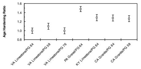
Figure 17. Average Age Hardening for Various Mixtures Subjected to Long-Term Oven Conditioning, as Calculated from Dynamic Modulus at 25 °C and 5 Hz Using the Field Shear Test (Error Bars are for Bonferroni Joint 95% Confidence Intervals).
