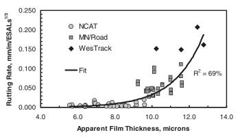
Figure 21. Relationship Between Rutting Rate and Apparent Film Thickness.
