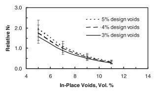
Figure 15. Effect of In-Place Air Voids and Design Air Voids on Relative In-Situ Fatigue Life (Errors Bars = 2s Confidence Limits).
