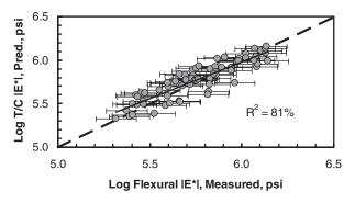
Figure 9. Predicted Complex Modulus in Tension/Compression Compared with Measured Flexural Complex Modulus for SHRP Mixtures (Bars = d2s Confidence Limits, Solid Line = Regression Function, and Dashed Line = Equality).
