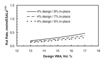
Figure 6. Effect of VMA and In-Place Air Voids on Rut Resistance of Superpave Mixtures at a Constant Design Air Void Content of 4%.
