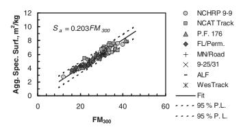
Figure 1. Estimated Aggregate Specific Surface as a Function of  $FM_{300} = P_{75} + P_{150} + P_{300}$  ( $r^2 = 90\%$ ; Plot Includes 95% Prediction Limits for New Observations).
