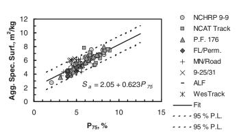
Figure 2. Estimated Aggregate Specific Surface as a Function of Material Finer than 75  $\mu$ m (r<sup>2</sup> = 76%; Plot Includes 95% Prediction Limits for New Observations).
