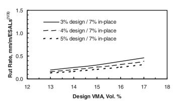
Figure 5. Effect of Design VMA and Air Voids on Rut Resistance of Superpave Mixtures at a Constant In-Place Air Void Content of 7%.
