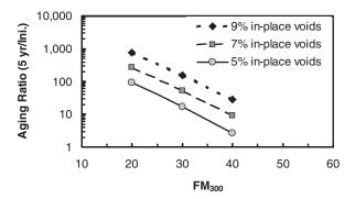
Figure 20. Predicted Binder Age-Hardening Ratio at 40 °C as a Function of In-Place Air Void Content and FM<sub>300</sub> for a MAAT of 15.6 °C.
