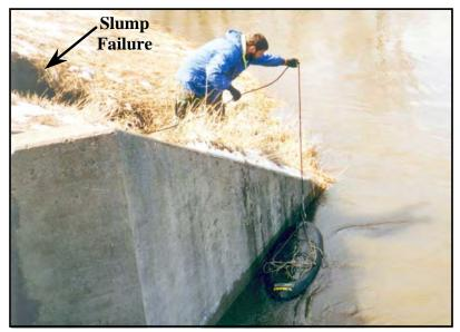
Figure 6. Scour measurement at upstream right wingwall of U.S. 12 bridge over the Pomme De Terre River; notice slump failure of embankment.
