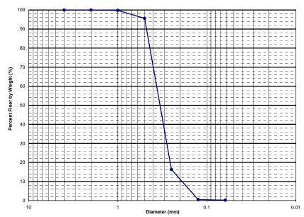
Figure 3. Grain size distribution for CR 22 bed material samples
