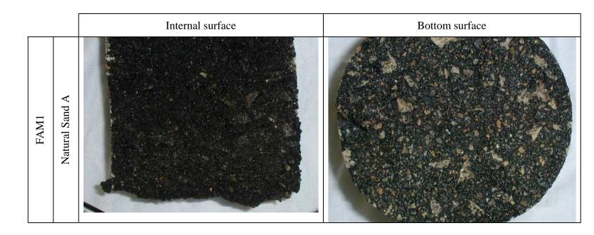
Figure E.6 Cores from FAM1 test section after traffic
