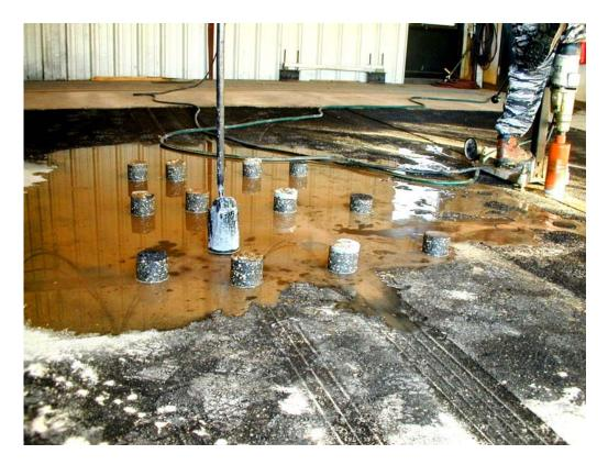
Figure D.9 Cores taken after traffic
