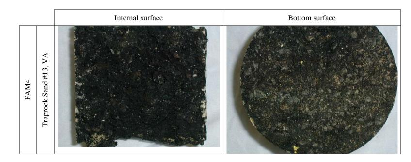
Figure E.9 Cores from FAM4 test section after traffic
