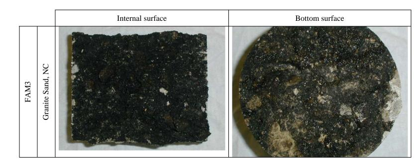
Figure E.8 Cores from FAM3 test section after traffic
