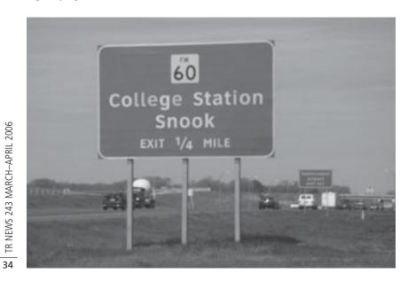
A 1994 study by the Federal Highway Administration (FHWA) found that guide signs did not provide adequate viewing distance and reaction time for older drivers. The report recommended enlarging the size of the letters on signs by 20 percent to increase the legibility distance.
