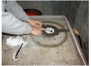
Figure 2-1. Applying Thermal Paste to Sensor
