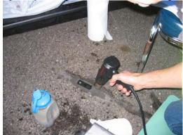
Figure 35. Drying a Pavement Sensor with a Heat Gun
