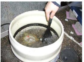
Figure 26. Laboratory Ice Bath - Vigorously Stirring Ice Bath Made with Distilled Water and Crushed Ice
