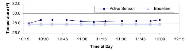
Figure 43. Graph Showing Active Sensor Stability over a Long Duration
