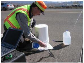
Figure 16. Cleaning a Pavement Sensor During the Field Surface State Test
