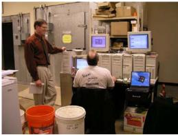
Figure 13. Data Acquisition System Outside Environmental Chamber Used in Laboratory Tests
