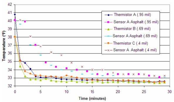
Figure 23. Laboratory Comparison of Different Plastic Bag Thicknesses
