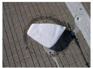
*Figure 6-2. Dry Ice Resting on Pavement Sensor.*
