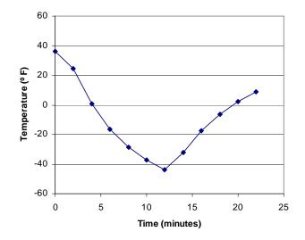
**Figure 34.** Graph Showing Temperature Recovery of a Sensor after the Dry Ice Test
