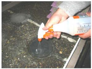
*Figure 3-2. Spraying Tap Water on Sensor Surface.*
