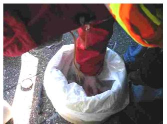
**Figure 22. Field Method for Establishing Ice Bath - Place Plastic Bag Over PVC Section** Part I: Final Report, page 54
