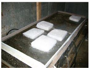
Figure 31. Dry Ice Cooling Asphalt Pavement Sensors
