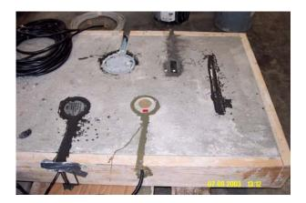
**Figure 9. Concrete Test Section after Sensor Installation**
