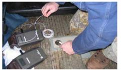
Figure 7. Applying Thermal Paste to Sensor.
