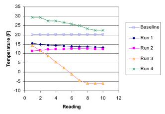
Figure 42. Passive Sensor Results with Sensor B using a 15 Percent Sodium Chloride Solution
