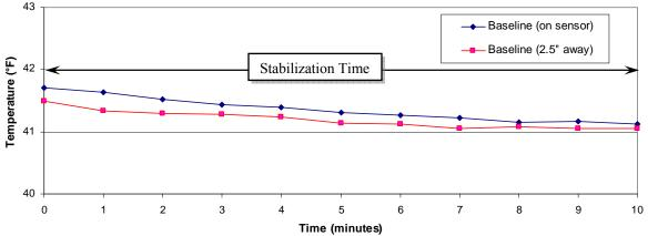
Figure 17. Graph of Time to Stabilize Pavement after Closing Environmental Chamber Door, Baseline Comparison
