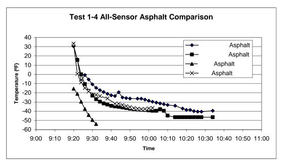
Figures G-8 and G-9. Comparison of sensor readings after dry ice was applied to sensor surface.
