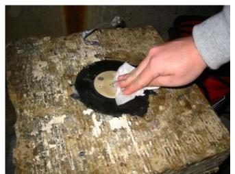
Figure 12. Active Sensor Embedded in a Separate Concrete Slab
