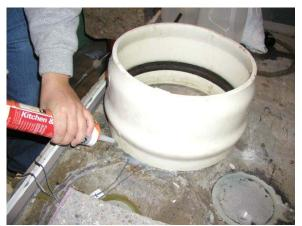
Figure 20. Laboratory Method for Establishing Ice Bath - Caulk PVC Pipe to Pavement Surface with Silicone
