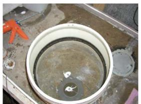
Figure 25. Laboratory Ice Bath -Unsecured Thermistors Do Not Stay In Place When Stirred
