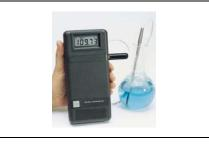
Thermometer and thermistor to check air/pavement temperature
