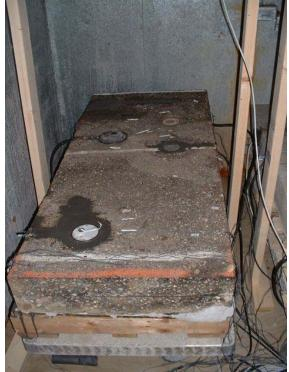
Figure 11. Asphalt Test Section Installed in Environmental Chamber
