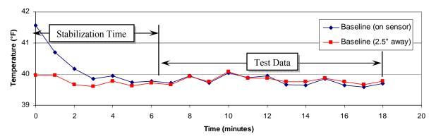
Figure 18. Graph Showing Effect of Water Film Cooling on the Pavement Section in Laboratory Test
