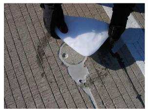
*Figure 6-1. Placing Dry Ice on Pavement Sensor.*
