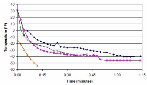
Figure 28. Laboratory Test – Temperature Comparison for Four Sensors Subjected to Dry Ice
