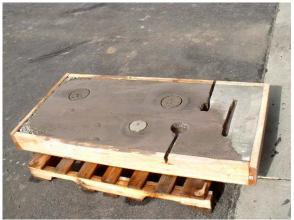
Figure 8. Concrete Core Drilling in Preparation for Sensor Installation
