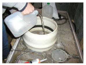
Figure 21. Laboratory Method for Establishing Ice Bath - Pour Distilled Water into Caulked PVC Pipe
