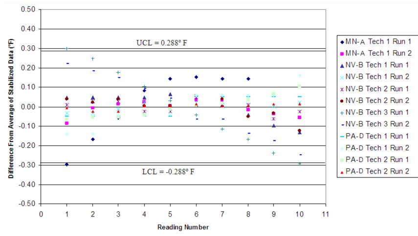
Figure 4. Run Chart for Statistical Process Control of Pavement Temperature for Field Tests
