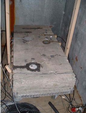
Figure 10. Concrete Test Section Installed in Environmental Chamber
