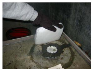
Figure 30. Applying Full 10" x 10" Block of Dry Ice to Pavement Sensor
