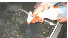
Figure 10. Spraying Tap Water on the Sensor Surface.
