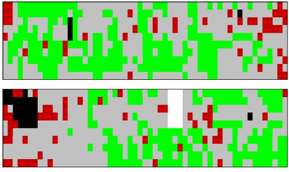
Figure A-8: Half-cell Potential Mapping for Bridge Deck of Structure located in Kentucky
