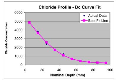
Figure 8: Curve Fit to ascertain "Apparent Diffusion Coefficient."
