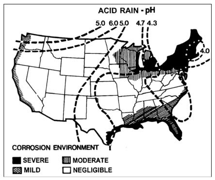
Figure 7: Corrosion environment of the US
