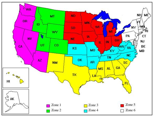
Figure 1: Delineation of zones based on corrosivity of the exposure conditions.
