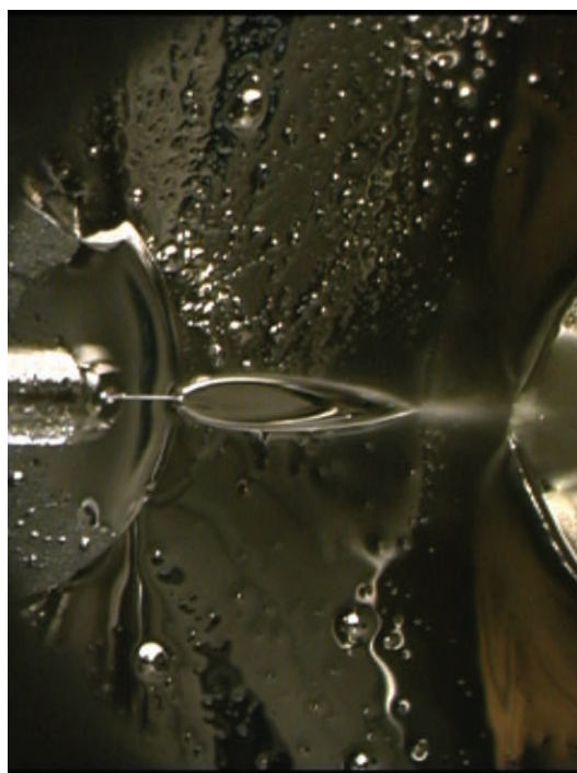
FIGURE 4.3 Layout of the liquid-lithium “foils” that serve as fragmentation targets for the heavy-ion beam from the accelerator. The foil on the left is 1 cm thick and 0.5 cm wide; it has been shown to be capable of serving as a target in a 400 kW beam. The foil on the right is the object in the center of the photograph. It is \sim 10^{-3} cm thick and has a high mass flow rate of 2 g/s. It is to be used to strip electrons from 10 MeV/A heavy-ion beams and should be able to handle the power deposition. Courtesy of Argonne National Laboratory, managed and operated by UChicago Argonne, LLC, for the U.S. Department of Energy under Contract No. DE-AC02-06CH11357.
