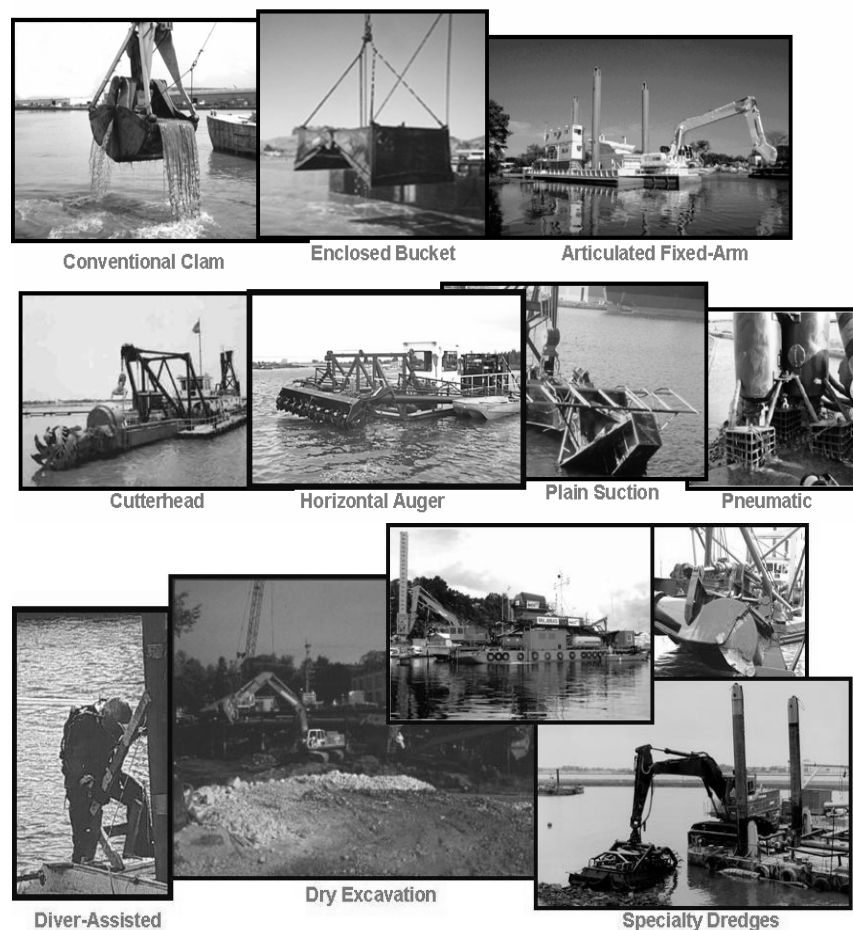
FIGURE 2-3 Categories of dredging and sediment removal equipment. Source: Francingues and Palermo 2006.
