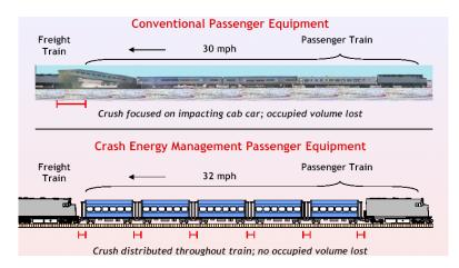
FIGURE 3 Train-to-train tests.
