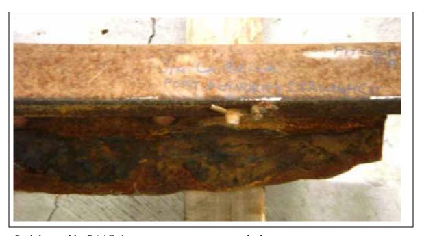
${\it Rail\ donated\ by\ PAAC\ showing\ severe\ corrosion\ at\ the\ base}.$
