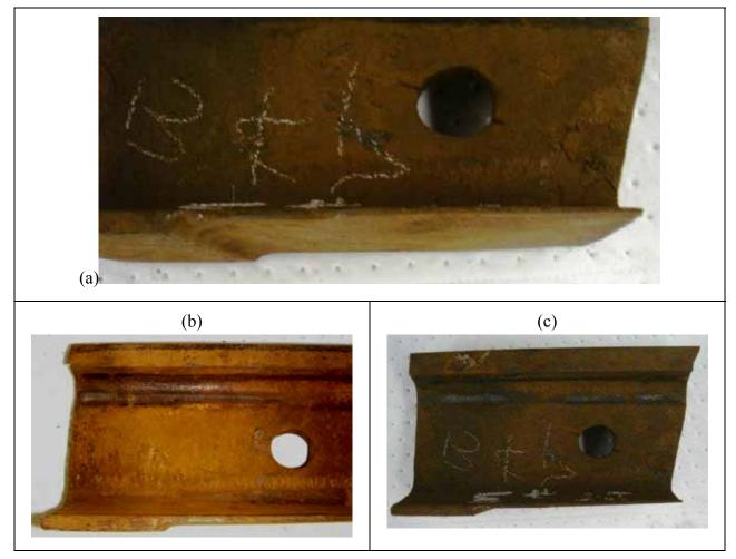
Figure 9. Pictures of the 136-lb rail donated from Amtrak for the rail base corrosion project showing a clear reduction from the base of the rail. Note: each transit authority has its own safety standard. However, most of them agree that a reduction in rail base between 1/8" to 1/4" is the maximum permissible allowance for immediate replacement of the rail.
