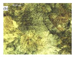
Figure 6. Microstructure of the 115-lb rail donated by the St. Louis, Missouri, Metro System. The sample in (a) as-polished, 500X and (b) as-etched conditions 1000 X, respectively.
