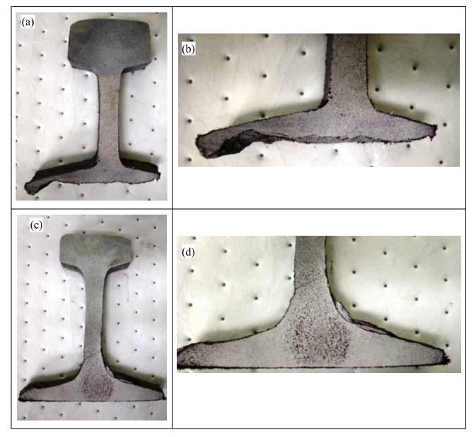
Figure 4. Pictures of the magnetic particles evaluation of the rail base for the Port Authority Trans-Hudson (a,b) and St. Louis, Missouri, Metro System (c,d). Note that there is no apparent evidence of cracks growing from the base of the rail to the parent material.
