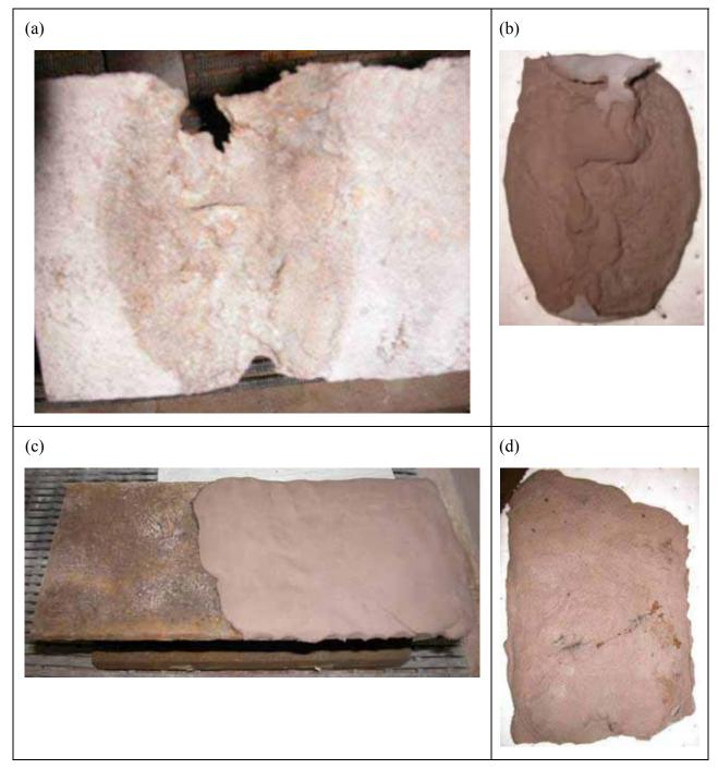
Figure 10. Pictures of the clay molds used to copy the detail and main features of the base of the rails for the numerical simulations. (a,b) 115-lb rail and (c,d) 136-lb rail.
