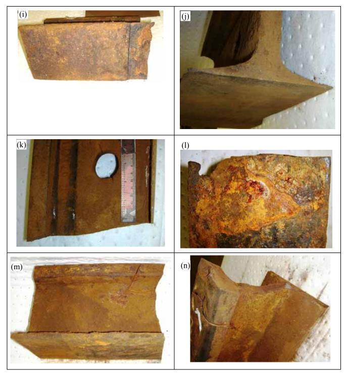
Figure 3 (continued). Sections of 136-lb rail showing different types of corrosion at the base of the rail. The presented macro-images of the rails show the rail donated by Amtrak. All of these rails failed due to corrosion in various locations along the east coast. The samples were used in the following way: (i) metallographic analysis, (j,k) numerical FEA simulations, (l,m,n) other examples. Note, view (i) shows one of the most severe corrosion conditions.
