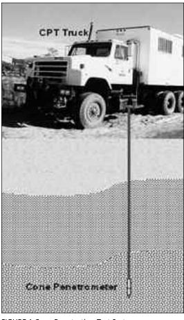
FIGURE 1 Cone Penetration Test System
