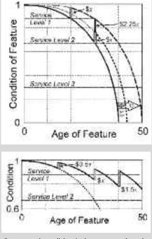
Conceptual condition index curve and service levels (top diagram); maintenance strategy scenario (bottom diagram).
