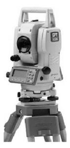
FIGURE 17 Total station survey device.
