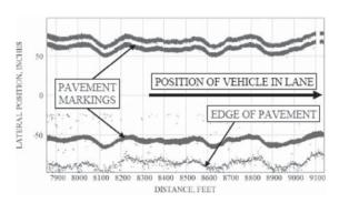
FIGURE 20 Lane wander measured by 360-degree scanning laser.
