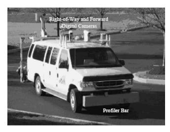
FIGURE 18 Road inventory vehicle with digital cameras and road profiling system (46).
