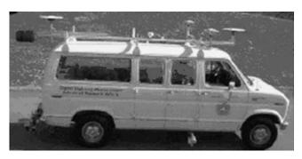
FIGURE 19 FHWA-Turner-Fairbank Highway Research Center digital highway measurement vehicle.
