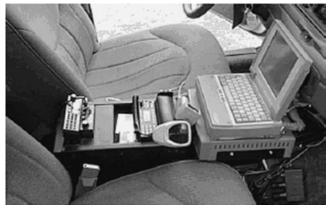
FIGURE 9 TraCS in-vehicle mobile data terminal (17).
