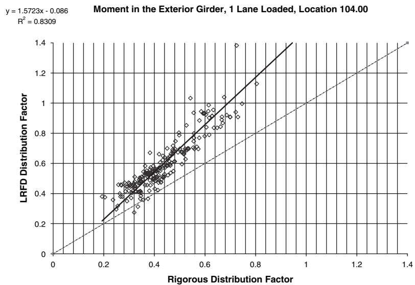
Figure 93. Slab-on-girder, moment, exterior girder, one lane loaded (example of a regression plot).
