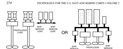
FIGURE 8.7 Integrated power system (right) advantage: Operators can determine how best to use the power, and the system saves 15 to 19 percent fuel in gas turbine surface combatants. SOURCE: Adapted from Krolick, C.F., 1996, "Advanced Surface Machinery Programs (ASMP)," presented to the Panel on Technology by the Naval Sea Systems Command, Arlington, Va., May 2.
