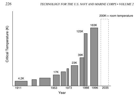
FIGURE 7.3 The increase over time in the critical superconducting temperature of HTS materials. SOURCE: Adapted from National Research Council, 1989, *Materials Science and Engineering for the 1990s: Maintaining Competitiveness in the Age of Materials*, National Academy Press, Washington, D.C., Figure 1.4, p. 23.
