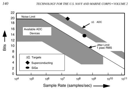
FIGURE 4.8 State-of-the-art analog-to-digital converters. Current development of Delta-Sigma ( $\Delta\Sigma$ ) devices will add up to 6 bits by the year 2000.
