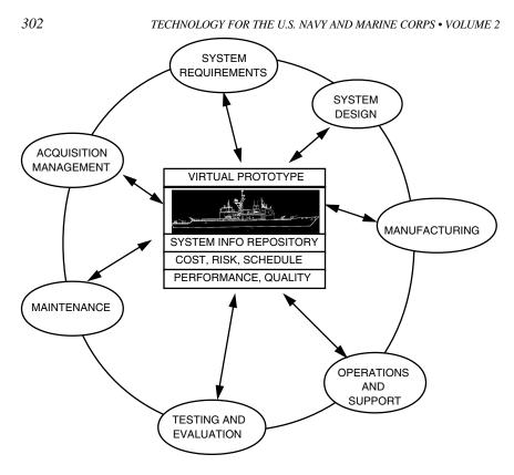
FIGURE 10.1 Schematic representation of the SBA process.
