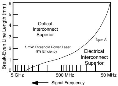
FIGURE 2.3 Break-even transmission line length—optical vs. electrical interconnect. SOURCE: Adapted from Cinato, P., and K.C. Young, Jr., 1993, "Optical Interconnections Within Multichip Modules," *Optical Engineering*, 32(4):852, April.
