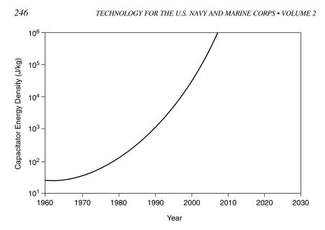
FIGURE 8.4 Projection of specific energy density for new capacitor technology. SOURCE: Adapted from the Board on Army Science and Technology, 1993, "Electric Power Technology for Battle Zones," *STAR 21: Strategic Technologies for the Army of the Twenty-First Century*, National Academy Press, Washington, D.C., Figure 43-4, p. 557.
