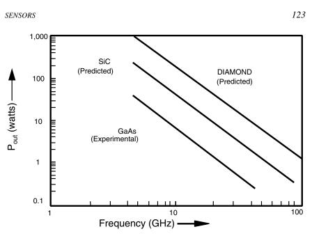
FIGURE 4.3 RF power performance vs. frequency for diamond, SiC, and GaAs MES-FETs. SOURCE: Adapted from Trew, Robert J., Jing-Bang Yan, and Philip M. Mock, 1995, "The Potential of Diamond and SiC Electronic Devices for Microwave and Millimeter Wave Power Applications," *Proceedings of the IEEE*, 79(5):598-620, Figure 15.
