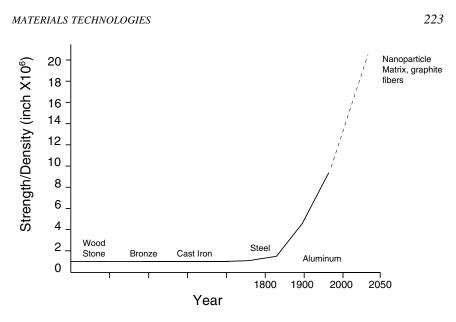
FIGURE 7.1 Tensile strength-to-density ratio of structural materials projected through 2035. The extrapolated values are based on a calculation of the maximum strength-todensity ratio of high-density single-crystal graphite fiber. SOURCE: Adapted from National Research Council, 1989, *Materials Science and Engineering for the 1990s: Maintaining Competitiveness in the Age of Materials*, National Academy Press, Washington, D.C., Figure 1.1, p. 20.
