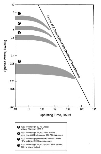
FIGURE 8.2 Specific power versus operating time for advanced turbogenerators. SOURCE: Adapted from the Board on Army Science and Technology, 1993, "Electric Power Technology for Battle Zones," *STAR 21: Strategic Technologies for the Army of the Twenty-First Century*, National Academy Press, Washington, D.C., Figure 43-1, p. 547.
