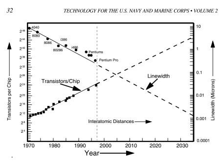
FIGURE 2.1 Microelectronic technology growth—fabrication linewidth and transistors per chip. SOURCE: Computation from data in Conrad, Michael, 1986, "The Lure of Molecular Computing," *IEEE Spectrum*, 23(10):55-60, October. See also information in Figures 4.2 and 4.7 in Chapter 4 of this report.
