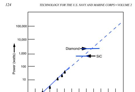
FIGURE 4.4 X-band power amplifier output. SOURCE: Adapted from the U.S. Air Force Scientific Advisory Board, 1995, *New World Vistas, Air and Space Power for the 21st Century, Sensors Volume*, U.S. Air Force, Washington, D.C., Figure 6-6, p. 102 and data shown in Figure 4.3 of this report.
