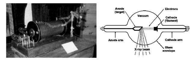
FIGURE B-8 (a) Photograph of Roentgen's apparatus for production of x-rays, referred to as Crookes cold cathode tube; (b) schematic diagram of a Coolidge tube, referred to as hot cathode tube.
