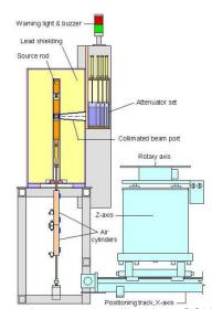
FIGURE 5-7 Typical gamma calibrator configuration for survey instrument calibration. SOURCE: Image provided by Hopewell Designs, Inc. (2007).
