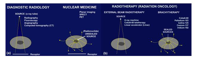
FIGURE B-9 Schematic diagram of ionizing radiation use in medicine for (a) diagnosis of disease (diagnostic radiology and nuclear medicine) and (b) treatment of disease (external-beam radiotherapy and brachytherapy). SOURCE: Provided by the committee.
