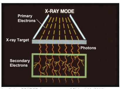
FIGURE 6-4 X-ray irradiation. SOURCE: Image courtesy of Cleland, M. (2006).
