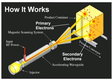
FIGURE 6-2 E-beam irradiation. SOURCE: Image courtesy of GAO (2002).
