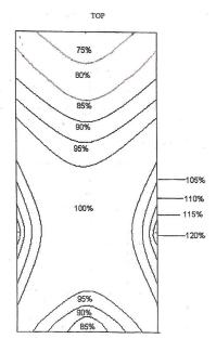
FIGURE 5-4 Typical dose map in a blood irradiation canister. SOURCE: Unpublished data on isodose curve in percentages for Gammacell 1000, provided by the American Red Cross, 2007.
