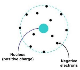
FIGURE B-1 Schematic diagram of the Rutherford atomic model. SOURCE: With kind permission of Springer Science+Business Media.
