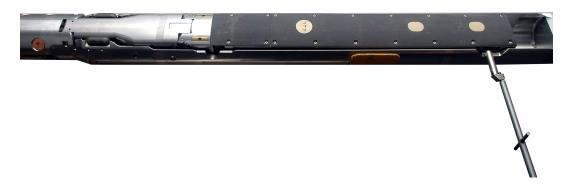
FIGURE 9-3 Atlas Densilog, which uses a vitrified cesium-137 source for wireline density measurements. The rod extending downward is a source handling device. The light-colored circles are windows for the source and detectors. SOURCE: Photo courtesy of Baker Hughes Inc.
