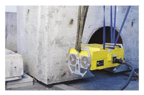
FIGURE 8-5 Photograph of an Inspecta betatron particle accelerator hanging in a harness and used for nondestructive examination. The x-ray energy can be varied from 2 MeV up to 6 MeV, which allows the radiographer to examine thick sections of steel or concrete. SOURCE: Copyright Inspecta.
