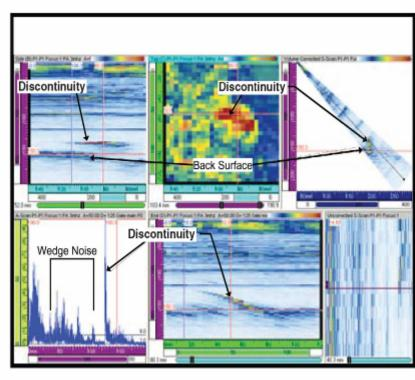
FIGURE 8-7 (a) Radiograph of a metal tube inside another larger metal tube. (b) Typical output from ultrasonic testing (of a different component) illustrating six panels of information obtained from the same component. SOURCE: (a) Blettner, A., et al. (2000), (b) Creech, M. (2006).
