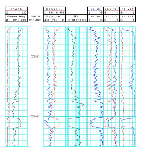
FIGURE 9-1 Typical logs and evaluation results from a string of well logging tools, including a natural gamma-ray log, a neutron log, an array induction log, and resistivity logs. The hydrocarbon volume result is also shown at the right. SOURCE: van Popta et al. (2004), courtesy of the Society of Petrophysicists and Well Log Analysts.
