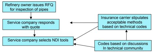
FIGURE 8-4 Process for selecting nondestructive testing method on the left, and factors that influence or dictate the process on the right. NOTE: RFQ = Request for quote. SOURCE: Provided by committee.
