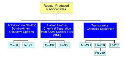
FIGURE 2-2 Origins of reactor-produced radionuclides for radiation sources. SOURCE: Adapted from Connell, et al. (2006).
