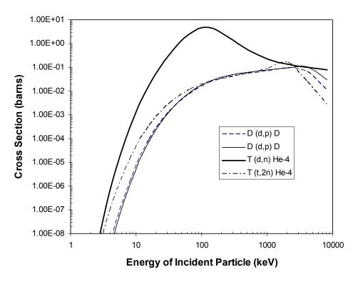
FIGURE 4-9 Fusion reaction cross sections as functions of kinetic energy. SOURCE: Image provided by the committee.
