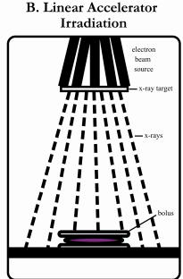
FIGURE 5-2 Diagrams of (A) a configuration of a gamma irradiator using cesium-137 and (B) a configuration of a linac irradiator. The plastic bolus is a container that enhances the dose uniformity in the irradiation configuration shown. SOURCE: Image provided by the committee.
