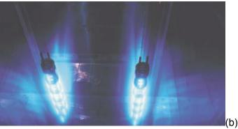
FIGURE 6-1 (a) An artist's rendition of an MDS Nordion JS-10000 panoramic irradiator, which uses a panel-type source rack (not necessarily to scale), and (b) a photograph of different source racks for an MDS Nordion Pallet Irradiator. SOURCE: Images courtesy of MDS Nordion (2002).
