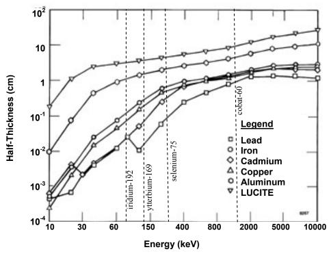
FIGURE 8-2 The half-value thickness (thickness that snields one-half of the incident photons) is shown for several common shielding materials. Each dashed line indicates the approximate location of the average energy for the gamma rays emitted by the radionuclide with which it is labeled. Note that the actual half-value is slightly higher for radionuclides that emit some higher-energy gamma rays, such as iridium-192. SOURCE: Adapted from ORTEC (2007).
