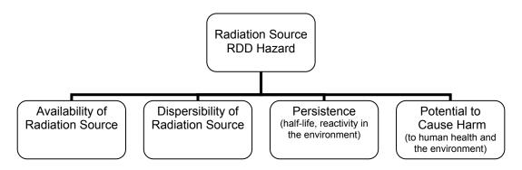
FIGURE 3-2 Key characteristics that make radiation sources hazardous with respect to area-denial RDDs. SOURCE: Image provided by the committee.
