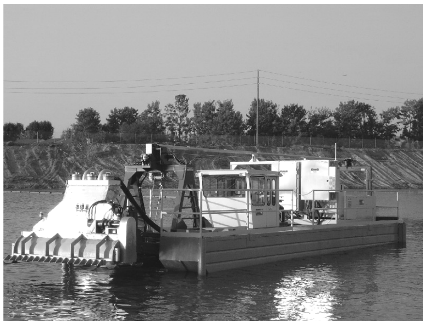
FIGURE 6-5 Basin cleaning vehicle (BCV) developed by Orange County Water District, California. This type of system allows clogging material to be removed while avoiding the water loss and expense associated with the downtime for draining and cleaning basins. Photo courtesy of Greg Woodside, Orange County Water District.
