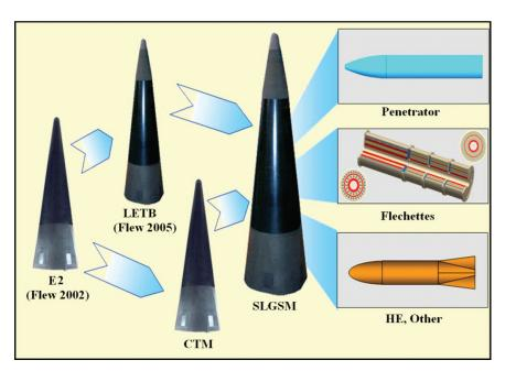
FIGURE 4-11 Relationship of the proposed Conventional Trident Modification (CTM) and Submarine-Launched Global Strike Missile (SLGSM) reentry bodies to the tested Enhanced Effectiveness (E2) Test Bed and Life Extension Test Bed (LETB) designs. The larger SLGSM would allow larger and more diverse payloads. SOURCE: Office of the Technical Director (Navy), Strategic Systems Programs, provided to the committee on December 18, 2007, Washington, D.C.
