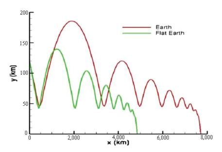
FIGURE G-1 Reentry trajectories for L/D = 2.2. Note that the last 1,000 km or more of the reentry trajectories are identical for Earth and flat Earth. SOURCE: Data for initial conditions (7 km/s,  $-10^{\circ}$  grazing) provided by G. Candler, University of Minnesota, personal communication to the committee, September 17, 2007.
