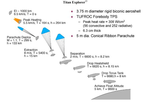
FIGURE 2.10 Illustration of the deployment sequence for the Titan Explorer airship. SOURCE: Courtesy of Joel S. Levine, NASA.
