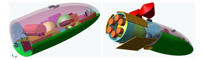
FIGURE 2.9 Illustration of a possible Neptune Orbiter mission utilizing aerocapture. The aerocapture stage is on the left; the coast stage, including two probes, is on the right. SOURCE: T.R. Spilker, Jet Propulsion Laboratory.
