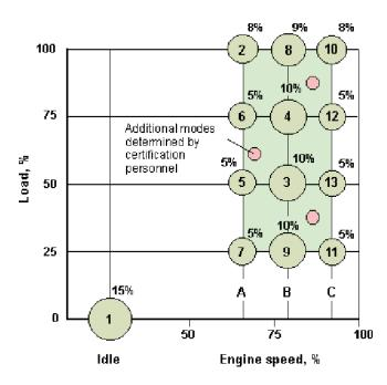
FIGURE 3-4 Thirteen-mode steady-state emission test conditions. SOURCE: DieselNet Online information service on clean diesel engines and diesel emissions. Available at www.dieselnet.com/standards/cycles/esc.html. Accessed August 6, 2007.
