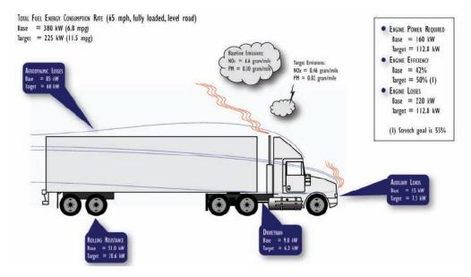
FIGURE 3-1 Energy audit of a typical Class 8 tractor-trailer combination on a level road at a constant speed of 65 mph and a GVW of 80,000 lb. SOURCE: DOE, 2006, p. 7.
