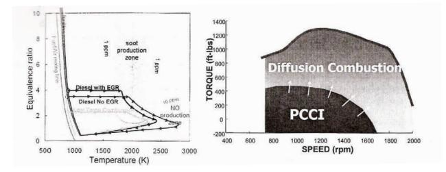
FIGURE 3-5 Illustration of the operating range for LTC combustion. SOURCE: Vinod K. Duggal, Cummins Engine Company, Inc., "Diesel Engine R&D and Integration," Presentation to the committee, Washington, D.C., February 9, 2007, Slide 14.
