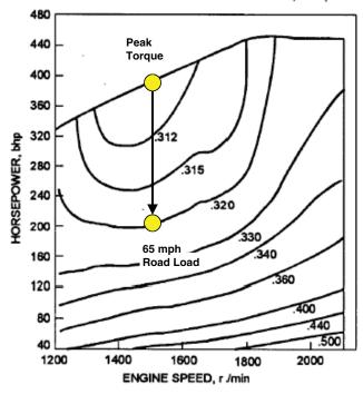
LINES OF CONSTANT FUEL CONSUMPTION, Ib/bhp + hr
