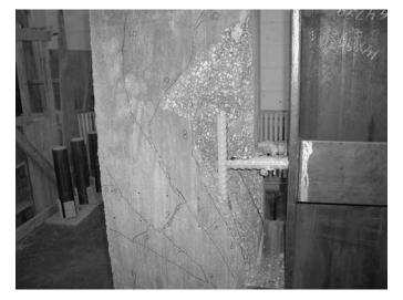
Figure 3.78. Concrete block push off in specimens without stirrups in the anchored hooked bar specimens.
