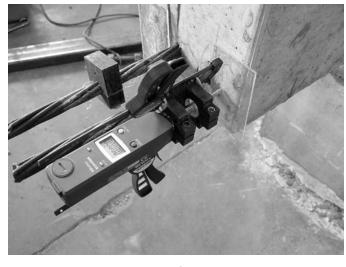
Figure 3.38. Mechanical deflection gage arrangement for measuring strand end slips at the beam end opposite to the test end.
