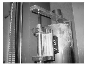
Figure 3.5. LVDT on NASP Test specimen.
