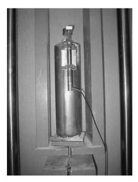
Figure 3.1. NASP specimen on the loading frame at OSU.
