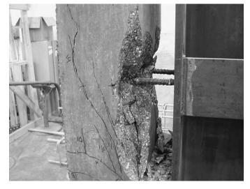
*Figure 3.79. Failure region in the case of Specimen III-13 with stirrups.*
