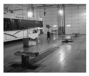
FIGURE 26 MTD hoist equipment for articulated buses.
