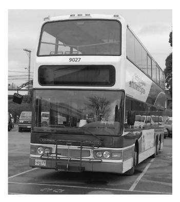
FIGURE 12 Low-floor double-deck bus of the Victoria Regional Transit System. (*Source*: BC Transit.)
