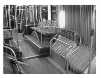
FIGURE 23 Hip rests used in MTD articulated buses.
