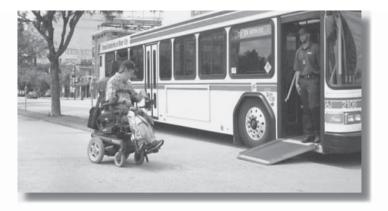
Wheelchair Access - Wheelchair lifts may be at the front or rear door, so bus stop designs need to allow for either possibility. Passengers in wheelchairs access the sidewalk/bus from a ramp deployed from the floor of the bus, which typically extends 2 to 3 feet from the edge of a bus to the curb.
