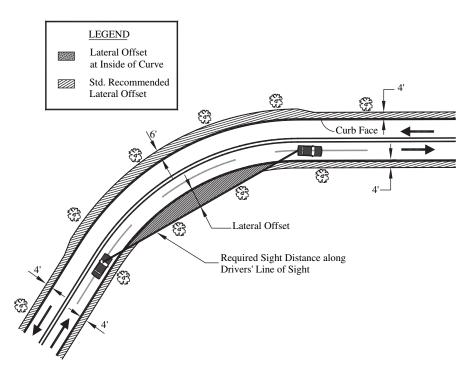
Figure C-1. Lateral placement of objects at horizontal curves.
