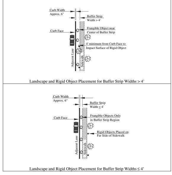
Figure 19. Object placement at buffer strips.
