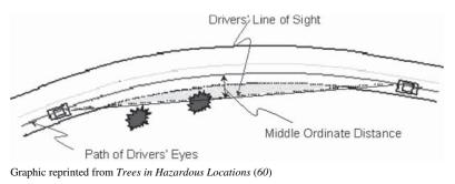
Figure 8. Sight distance around a horizontal curve.
