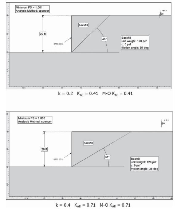
Figure 7-14A. SLIDE calibration analyses for horizontal backfill (homogeneous soil conditions).
