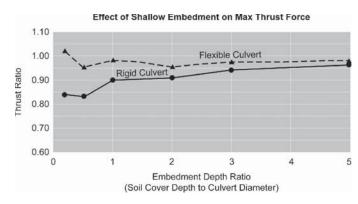
Figure 9-23. Embedment effects on culvert maximum thrust/hoop forces.
