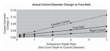
Figure 9-21. Culvert deformations versus free-field deformations.
