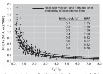
Figure 8-4. Normalized MHEA for deep-seated slide surface vs. normalized fundamental period of slide mass (Bray and Rathje, 1998).
