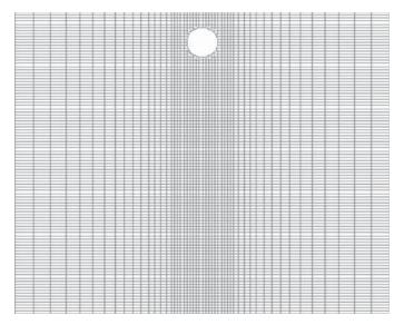
Figure 9-15. Case 5 finite difference mesh (soil cover = 5 feet).
