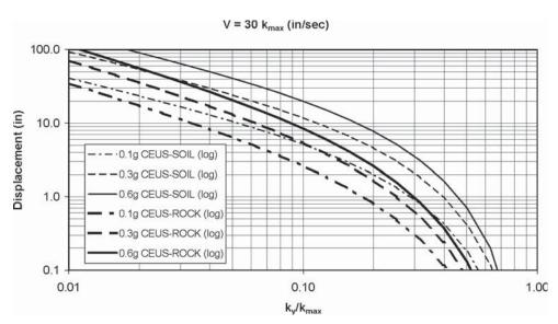
Figure 5-12. Comparison between CEUS-Rock and CEUS-Soil correlations for  $PGV = 30 \times k_{max}$ .
