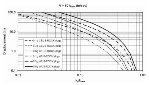
Figure 5-15. Comparison between WUS-Rock and CEUS-Rock correlations for  $PGV = 60 \times k_{max}$ .
