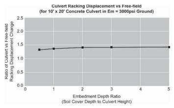
Figure 9-40. Racking ratios from FLAC analysis—Case 3.
