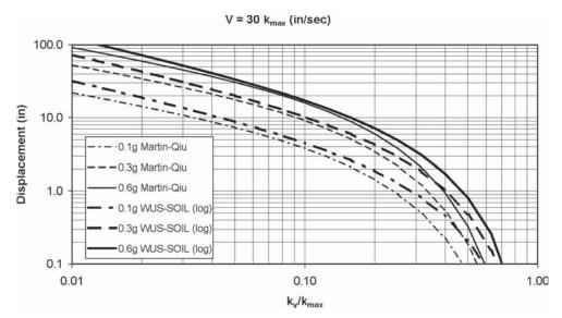
Figure 5-16. Comparison between Martin-Qiu and WUS-Soil correlations for  $PGV = 30 \times k_{max}$ .
