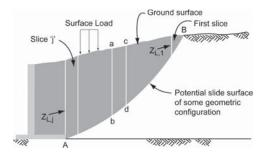
Figure 7-13. Adoption of slope stability programs to compute seismic earth pressure (Chugh, 1995).
