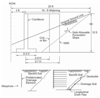
Figure 7-5. Cut slope construction.
