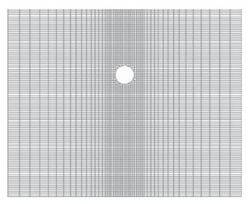
Figure 9-12. Case 2 finite difference mesh (soil cover = 30 feet).
