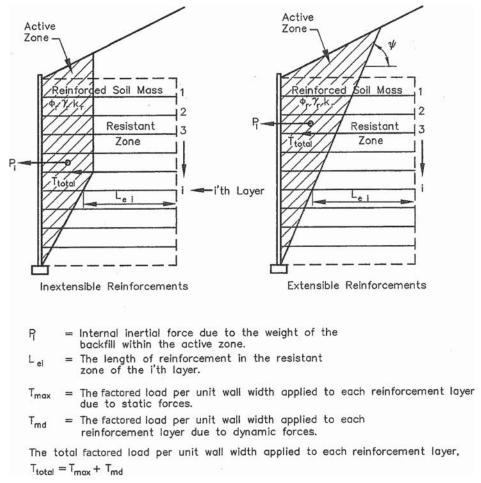
Figure 7-22. Seismic internal stability of a MSE wall (AASHTO, 2007).
