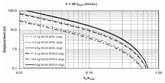
Figure 5-10. Comparison between WUS-Rock and WUS-Soil correlations for  $PGV = 30 \times k_{max}$ .
