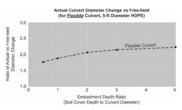
Figure 9-31. Ratios of culvert deformations versus free-field deformations (parametric analysis—Set 4).
