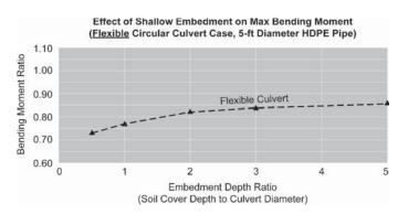
Figure 9-33. Embedment effects on culvert maximum bending moments (parametric analysis—Set 4).
