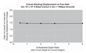
Figure 9-41. Racking ratios from FLAC analysis—Case 4.
