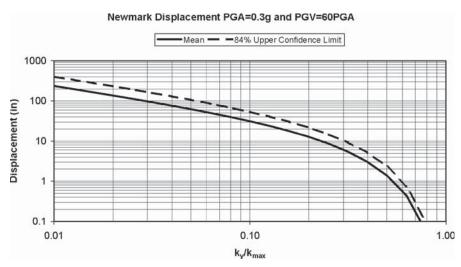
Figure 5-19. Mean Newmark displacement and 84% confidence level, PGA = 0.3g,  $PGV = 60 \times k_{max}$ .
