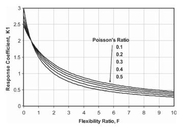
Figure 9-3. Seismic ovaling coefficient, K1.
