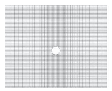
Figure 9-11. Case 1 finite difference mesh (soil cover = 50 feet).
