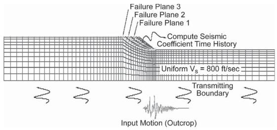
Figure 6-1. QUAD-4M model for 30-feet high wall.
