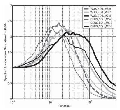
Figure 5-9. Average normalized spectral acceleration for soil records.
