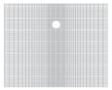
Figure 9-13. Case 3 finite difference mesh (soil cover = 20 feet).
