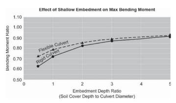
Figure 9-27. Embedment effects on culvert maximum bending moments (parametric analysis—Set 2).
