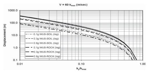
Figure 5-11. Comparison between WUS-Rock and WUS-Soil correlations for  $PGV = 60 \times k_{max}$ .
