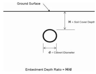
Figure 9-16. Definition of embedment depth ratio.
