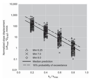
Figure 8-5. Normalized sliding displacement (SCEC, 2002; modified from Bray and Rathje, 1998).
