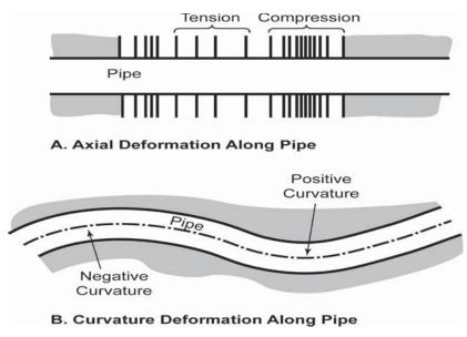
Figure 4-5. Axial/curvature deformations.
