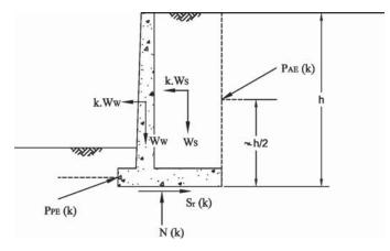
Figure 7-19. Seismic force diagram on retaining wall.
