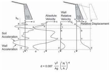
Figure 7-17. Concept of Newmark sliding block analysis (AASHTO, 2007).
