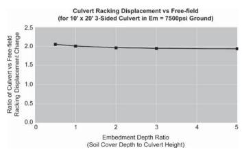
Figure 9-42. Racking ratios from FLAC analysis—Case 5.
