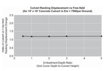
Figure 9-39. Racking ratios from FLAC analysis—Case 2.
