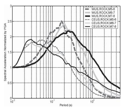
Figure 5-8. Average normalized spectral acceleration for rock records.
