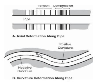
Figure 9-1. Axial and curvature deformations.
