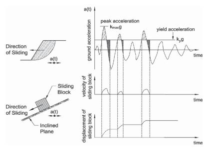
Figure 8-1. Newmark sliding block concept for slopes.
