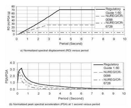
Figure 4-2. Spectral curve shapes for generic sites covering both WUS and CEUS (Sandia, 2004).
