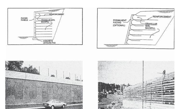
Figure 7-3. MSE wall types (after FHWA, 1996).
