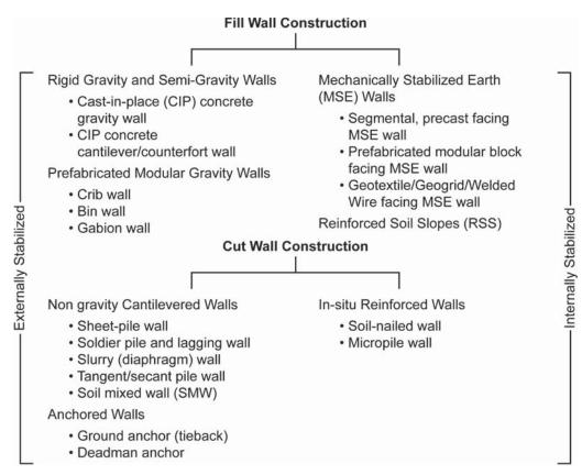
Figure 7-1. Earth retaining system classification (after FHWA, 1996).
