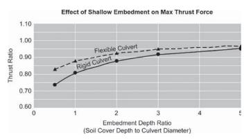
Figure 9-26. Embedment effects on culvert maximum thrust/hoop forces (parametric analysis—Set 2).
