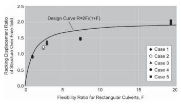
Figure 9-43. Recommended design racking curve.
