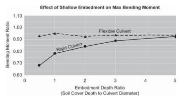
Figure 9-30. Embedment effects on culvert maximum bending moments (parametric analysis—Set 3).
