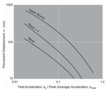
Figure 8-2. Permanent seismic deformation chart (Hynes and Franklin, 1984).
