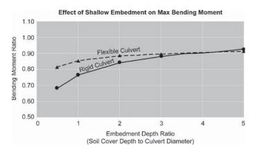
Figure 9-36. Embedment effects on culvert maximum bending moments (parametric analysis—Set 5).
