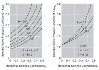
Figure 7-7. Effect of seismic coefficient and soil friction angle on active pressure coefficient.
