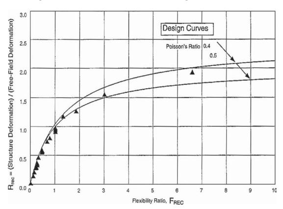
Figure 9-9. Racking ratio between structure and free-field.
