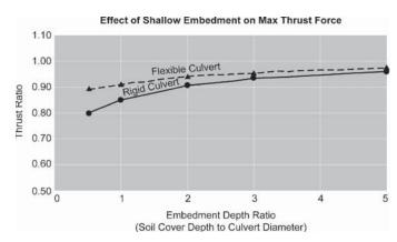
Figure 9-35. Embedment effects on culvert maximum thrust/hoop forces (parametric analysis—Set 5).
