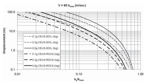
Figure 5-13. Comparison between CEUS-Rock and CEUS-Soil correlations for  $PGV = 60 \times k_{max}$ .
