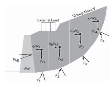
Figure 4-3. Limit equilibrium method for estimating seismic active earth pressures.
