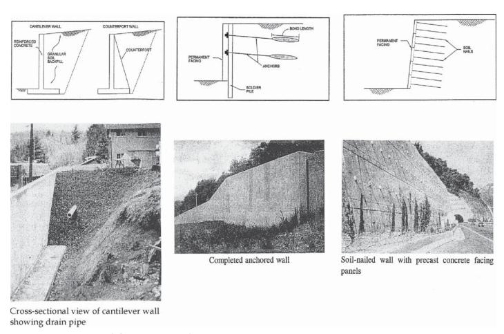
Figure 7-2. Wall types (after FHWA, 1996).
