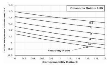
Figure 9-5. Seismic thrust/hoop force response coefficient,  $k_2$  (no-slip interface; soil Poisson's ratio = 0.35).
