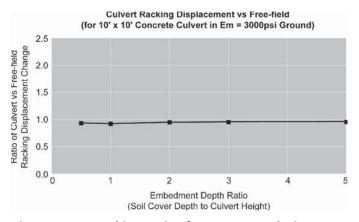
Figure 9-38. Racking ratios from FLAC analysis—Case 1.
