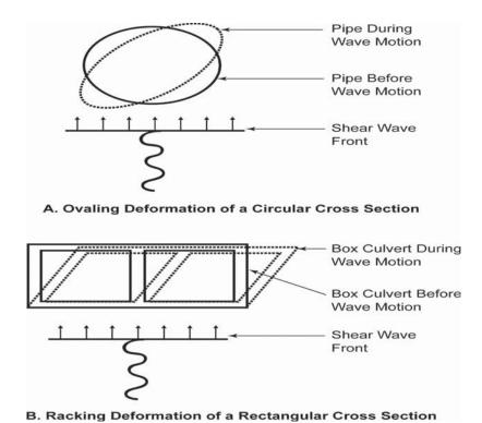
Figure 4-6. Ovaling/racking deformations.
