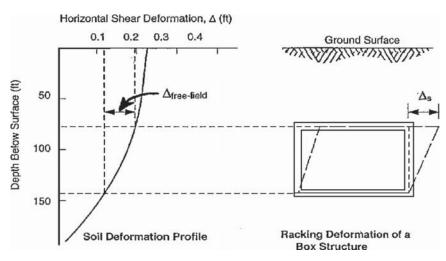
Figure 9-7. Racking deformations of a rectangular conduit.
