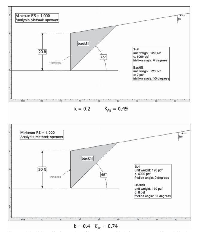
Figure 7-15B. SLIDE calibration analyses for sloping backfill (nonhomogeneous soil conditions).
