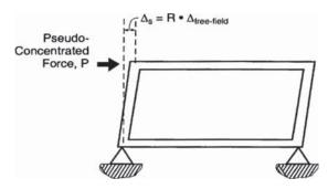
Figure 9-10. Simple frame analysis of racking deformations.
