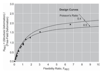
Figure 4-7. Earthquake-induced structural transient racking/ovaling deformations.
