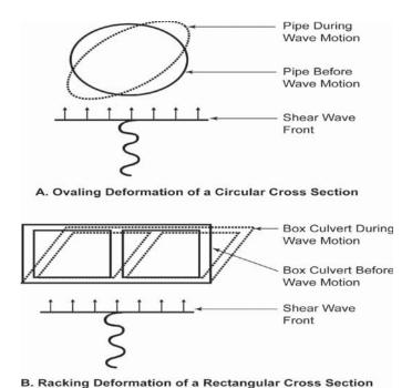
Figure 9-2. Ovaling and racking deformations.
