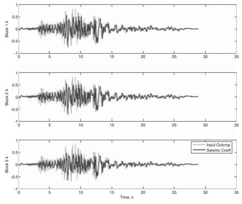
Figure 6-6. Scattering results for mid spectral shape, Imperial Valley EQ record.
