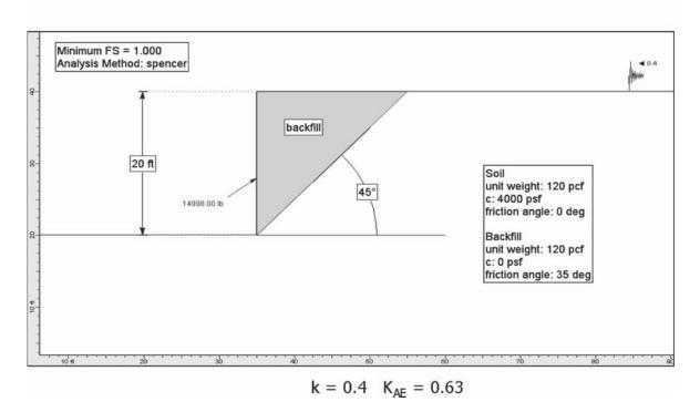
Figure 7-14B. SLIDE calibration analyses for horizontal backfill (nonhomogeneous soil conditions).
