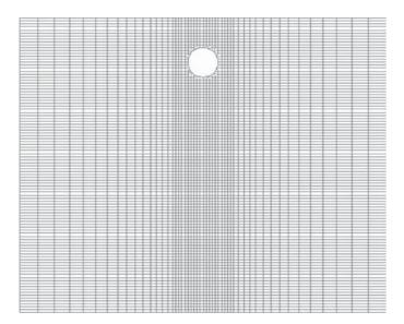
Figure 9-14. Case 4 finite difference mesh (soil cover = 10 feet).
