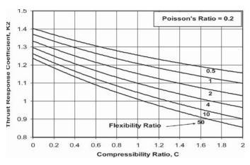
Figure 9-4. Seismic thrust/hoop force response coefficient,  $k_2$  (no-slip interface; soil Poisson's ratio = 0.2).
