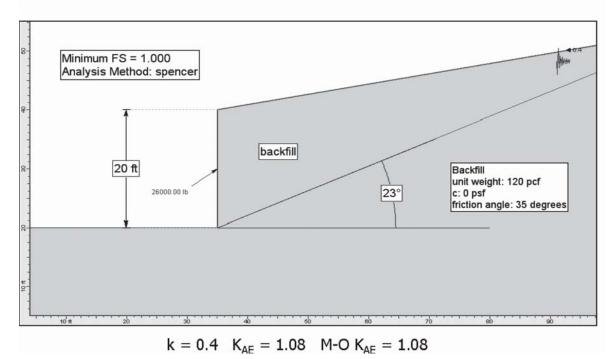
Figure 7-15A. SLIDE calibration analyses for sloping backfill (homogeneous soil conditions).
