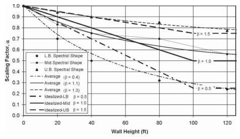
Figure 7-16. Simplified height-dependent scaling factor recommended for design.
