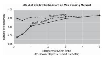
Figure 9-24. Embedment effects on culvert maximum bending moments.
