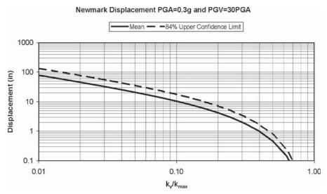
Figure 5-18. Mean Newmark displacement and 84% confidence level, PGA = 0.3g,  $PGV = 30 \times k_{max}$ .
