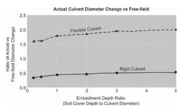
Figure 9-22. Ratios of culvert deformations versus free-field deformations.
