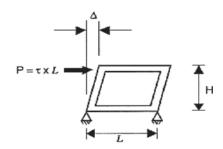
B. Flexural (Racking) Distortion of a Rectangular Frame
