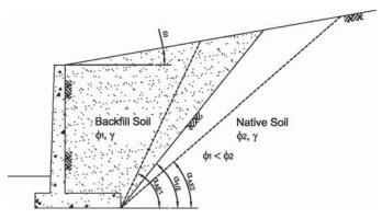
Figure 7-10. Application of M-O method for nonhomogeneous soil.
