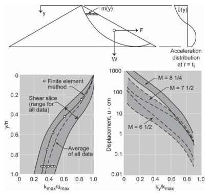
Figure 8-3. Permanent seismic deformation charts (Makdisi and Seed, 1978).
