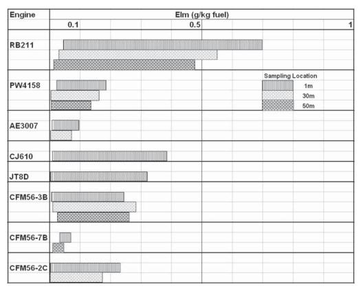
Figure D1.7. Ranges of measured mass-based emission index for engines emissions sampled in the near field plume.
