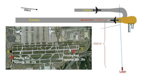
*Figure 6. Schematic of layout of mobile laboratories during the downwind study at Delta Atlanta-Hartsfield.*
