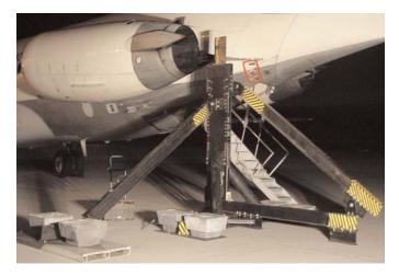
Figure 5. Probe rake assembly used during Phase 1 of the Delta Atlanta-Hartsfield Study.
