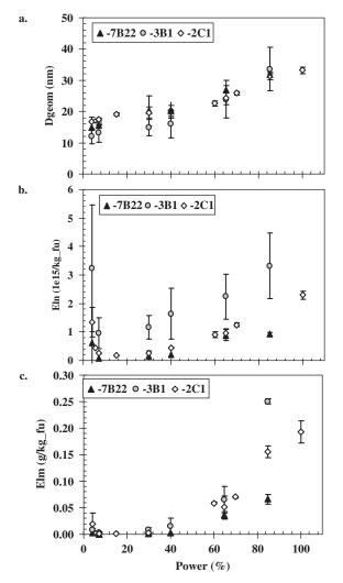
Figure D1.4. Mean particle diameter, number-based emission index, and mass-based emission index as a function of engine power for the -2C1, -3B1, and -7B22 models of the CFM56 class of engines.
