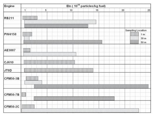
Figure D1.6. Ranges of measured number-based emission index for engines emissions sampled in the near field plume.
