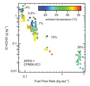
Figure D2.4. Formaldehyde emission index (EI) as a function of fuel flow rate measured during APEX1 for a CFM56-2C1 engine. Power condition is indicated directly on the graph.
