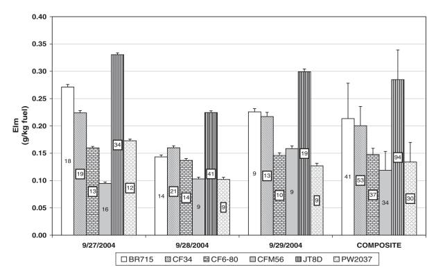
Figure D1.3. Average mass-based emission indices at take-off measured for six aircraft engine families during the Delta-Atlanta Hartsfield Study.
