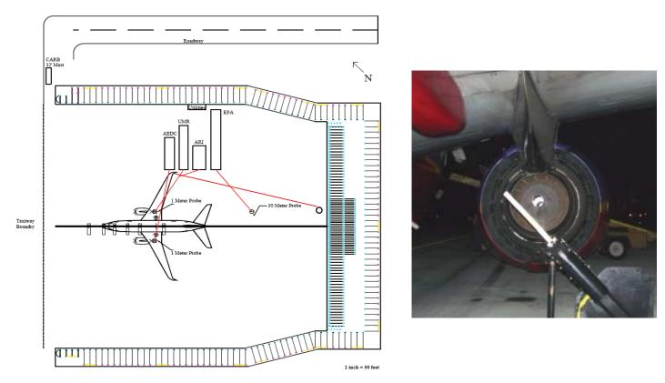
Figure 7. Layout of the mobile laboratories in the GRE and probe rake assembly used in JETS-APEX2.
