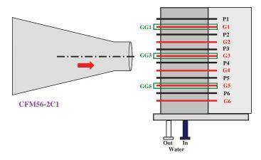
Figure 4. Orientation of sampling probes (P-particulate, G-gaseous, GG-external gaseous) with respect to the engine exit plane.
