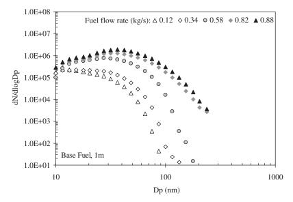
*Figure D1.1. Typical particle size distributions. Source:* Lobo, Hagen, Whitefield, and Alofs, "Physical Characterization of Aerosol Emissions from a Commercial Gas Turbine Engine." *Journal of Propulsion and Power*, 2007, 23 (5), p. 922.
