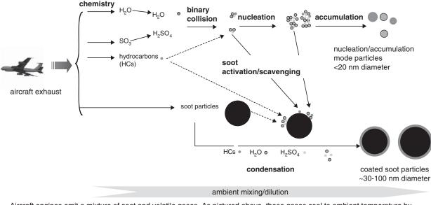
Aircraft engines emit a mixture of soot and volatile gases. As pictured above, these gases cool to ambient temperature by mixing with ambient air and convert to the particle phase by condensation and nucleation/growth. The nucleation/growth mode particles and soot coatings are complex mixtures of sulfuric acid, water, partially burned hydrocarbons, and engine oil.
