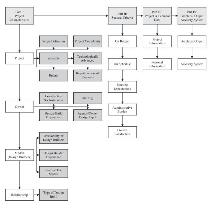
FIGURE 17 Design-build selector flowchart.
