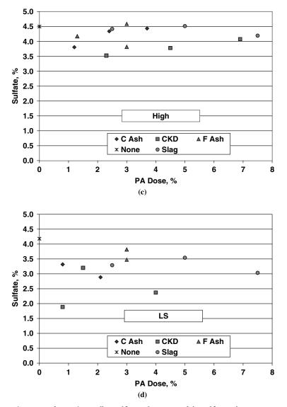
Figure 6. (Continued). Sulfate dosages. (c) Sulfate dosage required for optimization for High C<sub>3</sub>A Clinker as a function of Processing Addition type and dosage. (d) Sulfate dosage required for optimization for Mid-range C<sub>3</sub>A Clinker with limestone as a function of Processing Addition type and dosage.
