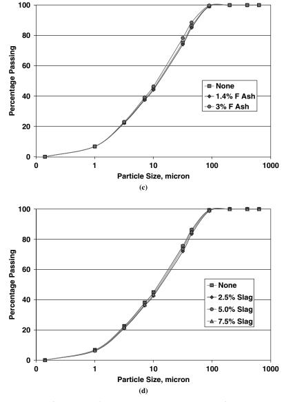
Figure 5. (Continued). Particle size distributions of selected cements without supplementary cementing materials. (c) PSD curves for low clinker with Class F Ash processing addition. (d) PSD curves for low clinker with slag processing addition. (continued on next page)
