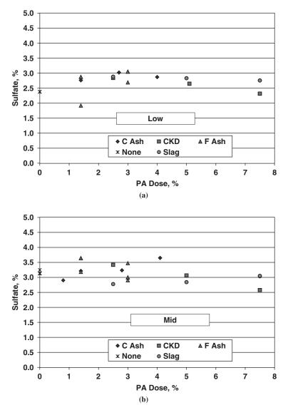
Figure 6. Sulfate dosages. (a) Sulfate dosage required for optimization for Low C<sub>3</sub>A Clinker as a function of Processing Addition type and dosage. (b) Sulfate dosage required for optimization for Mid-range C<sub>3</sub>A Clinker as a function of Processing Addition type and dosage.
