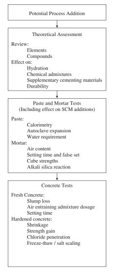
*Figure 2. Flow diagram of experimental work.*
