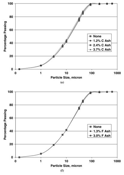
Figure 5. (Continued). Particle size distributions of selected cements without supplementary cementing materials. (e) PSD curves for high clinker with Class C Fly Ash processing addition. (f) PSD curves for high clinker with Class F Fly Ash processing addition.
