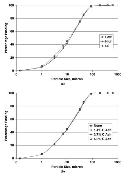
Figure 5. Particle size distributions of selected cements without supplementary cementing materials. (a) PSD curves for clinkers without processing additions. (b) PSD curves for low clinker with Class C Ash processing addition.
