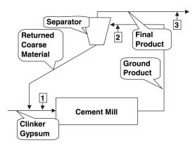
*Figure 1. Schematic illustration of cement grinding circuit. Note: Processing additions may be added to the material flow at Points 1, 2, or 3.*
