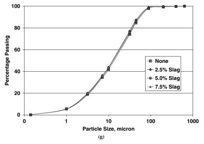
Figure 5. (Continued). Particle size distributions of selected cements without supplementary cementing materials. (g) PSD curves for high clinker with slag processing addition.
