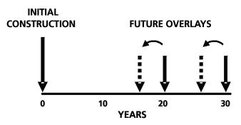
FIGURE 2 Diagram showing consequences of premature failure.
