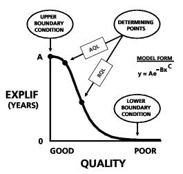
FIGURE 1 Diagram of performance-modeling technique. (EXPLIF = expected service life; AQL = acceptable quality level; RQL = rejectable quality level.)
