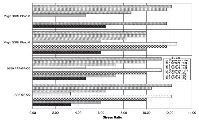
Figure 4.11. Stress ratios for dry and wet triaxial tests on RAP and virgin samples.
