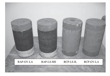
Figure 4.16. Molded RAP and RCP samples.
