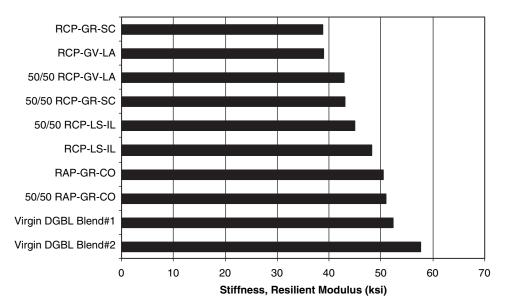
Figure 5.17. Estimated stiffness at 100 psi bulk stress (sat. repeated load triaxial test).
