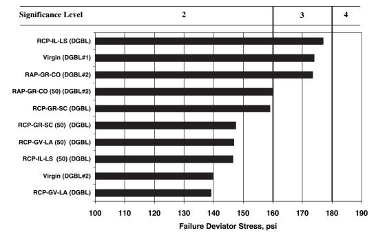
Figure 5.22. Performance potential based on repeated load triaxial test (saturated).
