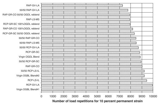
*Figure 4.13. Number of load repetitions at 10-percent permanent strain (dry tests).*
