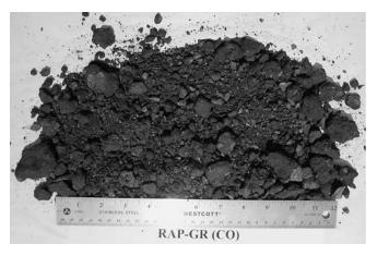
*Figure 3.11. Photograph of RAP-GR-CO material used for laboratory testing.*
