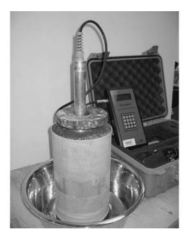
Figure 4.17. Apparatus used to make surface dielectric measurements.
