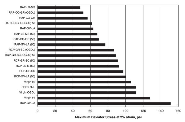
Figure 5.11. Shear strength at 2-percent strain in repeated load triaxial test.
