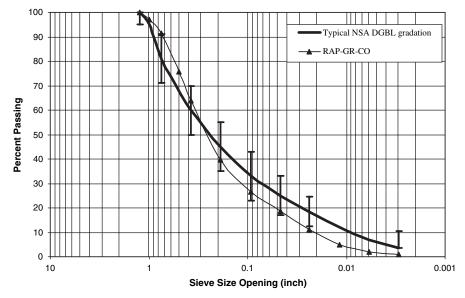
*Figure 3.10.* RAP-GR-CO as-received gradation and typical NSA DGBL gradation.
