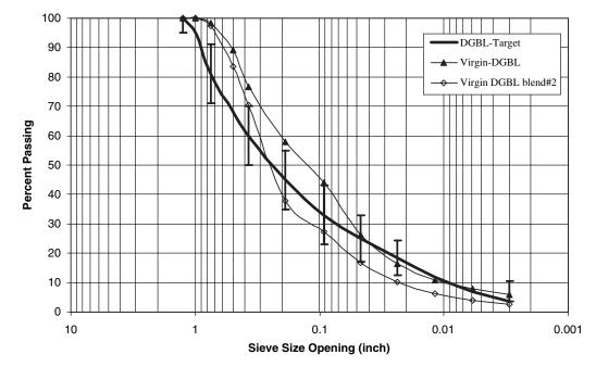
Figure 4.4. Gradation results of virgin aggregate DGBL-blended sample.
