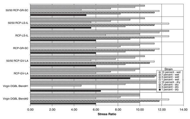
Figure 4.12. Stress ratios for dry and wet triaxial tests on RCP samples.
