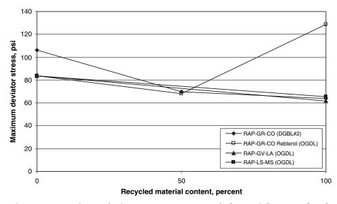
Figure 5.4. Maximum deviator stress versus recycled material content (RAP).
