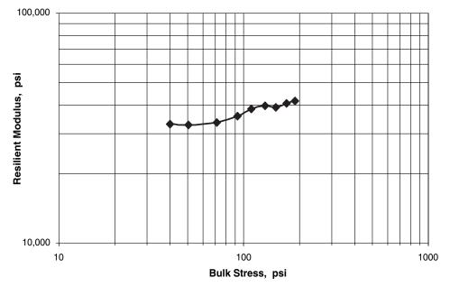
Figure 4.15. Resilient modulus test results for RCP-GR-SC.
