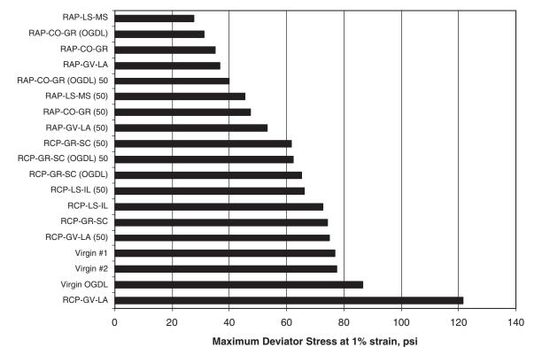
Figure 5.10. Shear strength at 1-percent strain in repeated load triaxial test.
