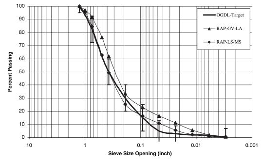
Figure 4.2. Gradation results of RAP as-received OGDL samples.
