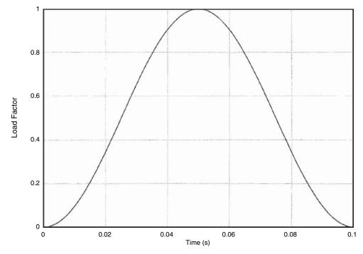
Figure 3.1. Load pulse for repeated load triaxial tests.
