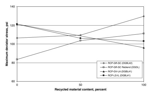
Figure 5.5. Maximum deviator stress versus recycled material content (RCP).
