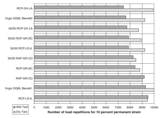
Figure 4.14. Failure load repetitions for wet and dry tests.
