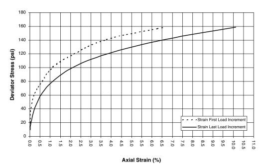
Figure 4.7. Repeated load triaxial test results for RCP-GR-SC at OMC.
