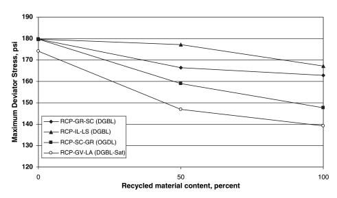
Figure 5.8. Repeated load triaxial test results for RCP samples.
