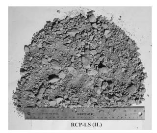
Figure 3.3. Photograph of RCP-LS-IL material used in laboratory testing.
