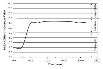
*Figure 4.18. Dielectric constant value curve with time for RCP-GV-LA.*
