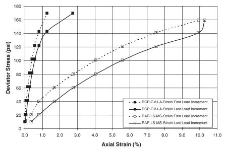
*Figure 5.14.* Comparison of load/unload curves for typical RCP and RAP materials.
