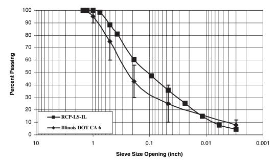
Figure 3.2. RCP-LS-IL as-received gradation and typical Illinois DOT CA 6 gradation.
