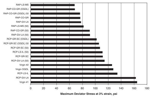
Figure 5.12. Shear strength at 3-percent strain in repeated load triaxial test.
