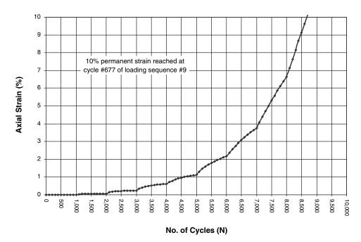
*Figure 4.8. Load repetitions versus permanent axial strain for RCP-GR-SC at OMC.*
