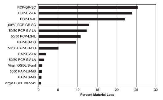
Figure 5.2. Canadian Freeze-Thaw test results.
