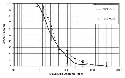
*Figure 4.5. Gradation results of virgin aggregate OGDL-blended sample.*
