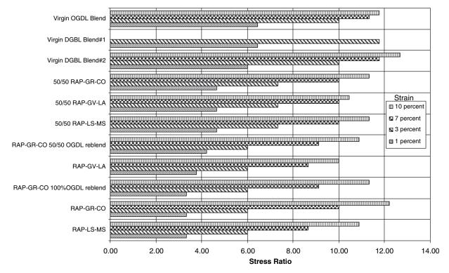
Figure 4.9. Stress ratios for dry triaxial tests on RAP samples.
