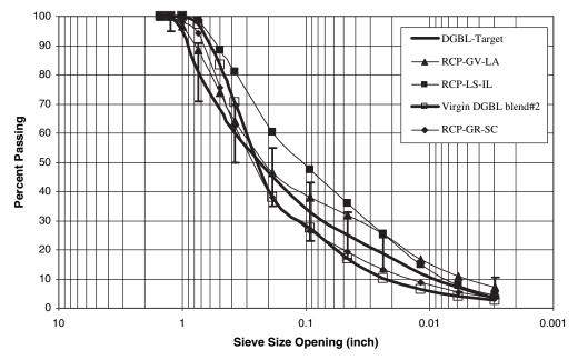
Figure 4.1. Gradation results of RCP as-received DGBL samples.
