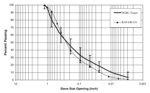
Figure 4.3. Gradation results of as-received RAP DGBL samples.
