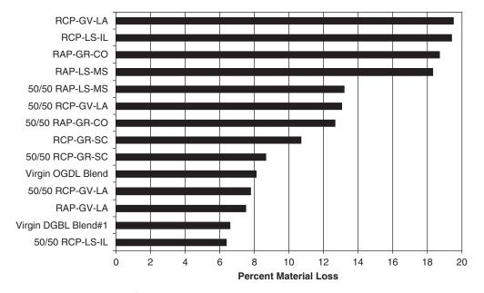
Figure 5.1. Results of Micro-Deval tests.
