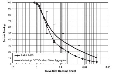
Figure 3.8. RAP-LS-MS as-received and Mississippi DOT aggregate gradations.
