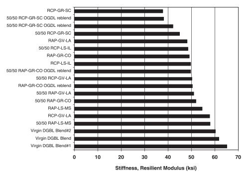
*Figure 5.16. Stiffness estimate using repeated load triaxial data at 100 psi bulk stress.*
