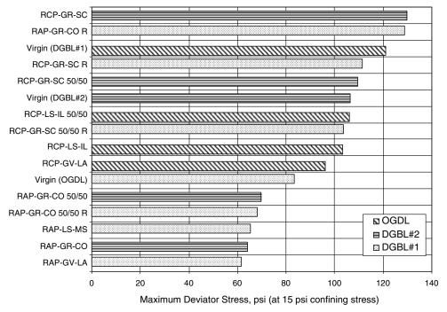
Figure 4.6. Maximum deviator stress in static triaxial tests.
