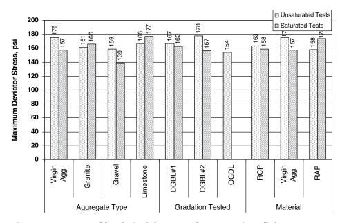
Figure 5.6. Repeated load triaxial test results at 15 psi confining pressure.
