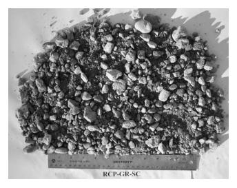
*Figure 3.7. Photograph of RCP-GR-SC material used in laboratory testing.*
