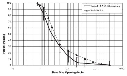
Figure 3.12. RAP-GV-LA as-received and typical NSA OGDL gradation.
