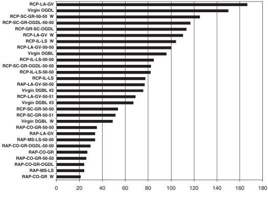
Initial Slope (percent change in deviator stress per unit permanent strain)
