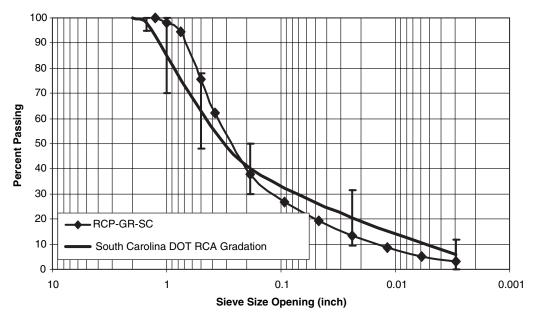
Figure 3.6. RCP-GR-SC as-received gradation and typical SC DGBL gradation.
