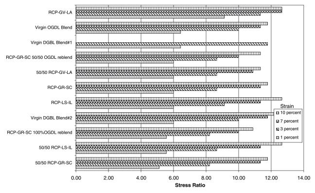
Figure 4.10. Stress ratios for dry triaxial tests on RCP and virgin samples.
