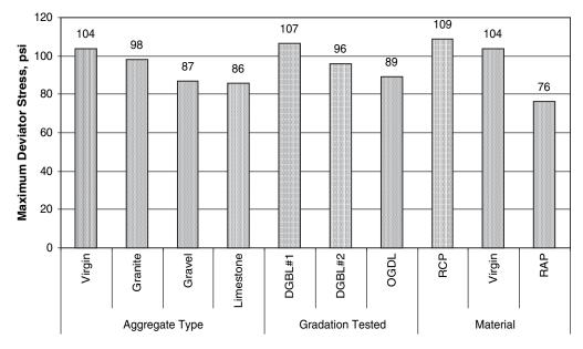
Figure 5.3. Static triaxial test results at 15 psi (103.4 kPa) confining pressure.
