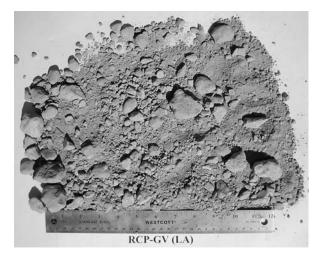
Figure 3.5. Photograph of RCP-GV-LA material used in laboratory testing.
