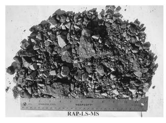
*Figure 3.9. Photograph of RAP-LS-MS material used for laboratory testing.*
