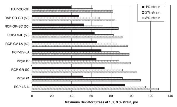
Figure 5.13. Shear strength materials tested saturated in repeated load triaxial test.
