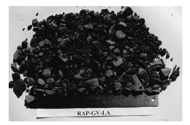
*Figure 3.13. Photograph of RAP-GV-LA material used for laboratory testing.*
