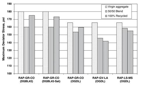
Figure 5.7. Repeated load triaxial test results for RAP samples.
