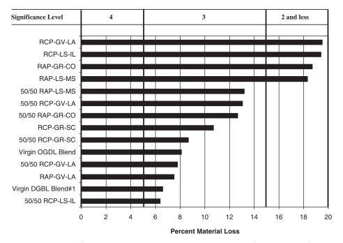
Figure 5.18. Performance potential based on toughness (Micro-Deval) test.
