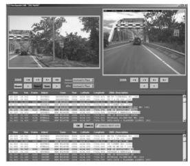
Incremental Index and Editor's linear-referencing screen shows the 2005 image (right) with the 2006 image proposed for a checkpoint.
