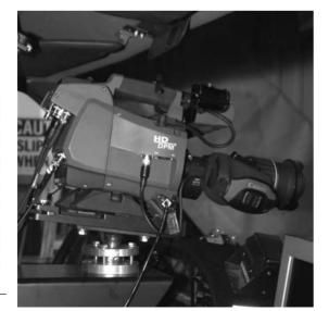
mize the imaging. Connecticut DOT and CTI selected the Thomson Grass Valley Worldcam LDK 6000 MK II for evaluation. The camera captures progressive-scan high-definition images with three 9.2-million pixel, high-definition, charge-coupled devices in
