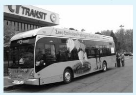
CT Transit, which provides public transit for Hartford, New Haven, and Stamford, Connecticut, has tested a hybrid passenger bus that uses a zero-emission hydrogen fuel cell.
