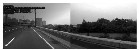
Dual camera views from the old camera system (above), compared with single HD image of the same roadway segment (below).
