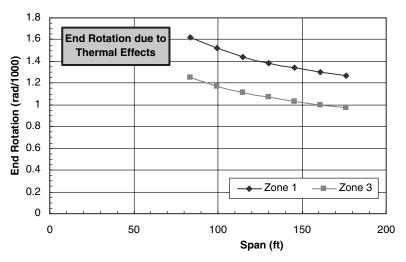
Figure 2.19. Rotation due to thermal gradient on girder.
