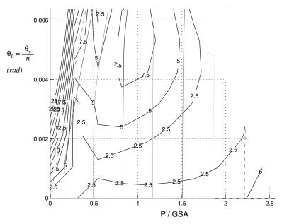
Figure 2.13. Iso-error plot (in %) for shear strain,  $\gamma_{zx}$ . Bearing with S=9 and no external plates, based on a fourth-order fit. (Constructed for Shear Strain at  $\frac{1}{4}$  in. Distance from the Critical Edge of the Shim).
