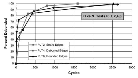
Figure 2.5. Debonding for PLT test series.
