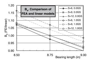
Figure 2.9. Stiffness coefficient B<sub>a</sub> for various S, based on various definitions of L.
