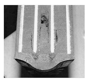
Figure 2.3. Internal damage caused by severe cyclic loading.
