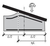
Figure 2.15. Lift-off: bearing behavior assumed in "semilinear" model.
