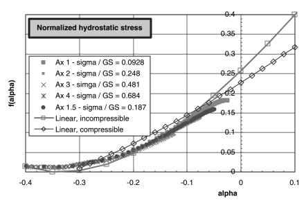
Figure 2.11. Hydrostatic stress: comparison between linear theory and FEA results.
