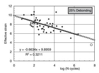
Figure 2.17. Effective strain vs. number of cycles: 25% debonding.
