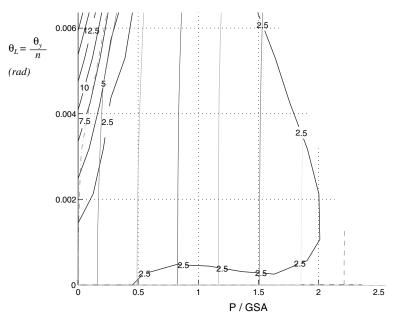
Figure 2.12. Iso-error plot (in %) for shear strain,  $\gamma_{zx}$ . Bearing with S=9 and bonded external plates, based on a fourth-order fit. (Constructed for Shear Strain at  $\frac{1}{4}$  in. Distance from the Critical Edge of the Shim).
