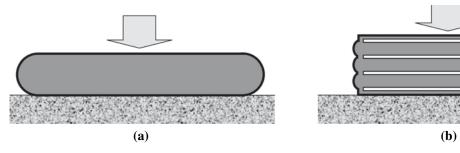
Figure 1.3. Bulges without (a) and with (b) steel plates.
