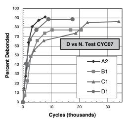
Figure 2.4. Progression of debonding with increased load cycles.
