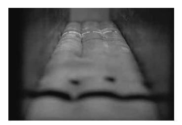
Figure 2.2. Initial debonding of bearing.
