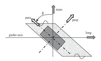
Figure 3.2. Orientation of axes for skew bridge.
