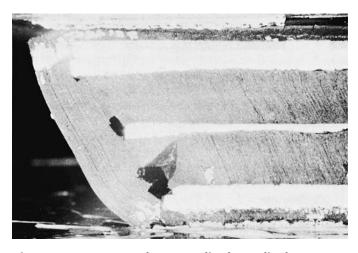
Figure 2.6. Damage due to cyclic shear displacements (from NCHRP Report No. 298).
