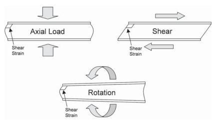
Figure 1.4. Deformations of a laminated elastomeric bearing layer.
