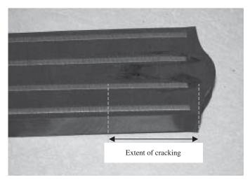
Figure 2.16. Shear crack propagation into elastomer layer.
