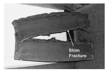
Figure 1.6. Fractured steel plates in bearing.
