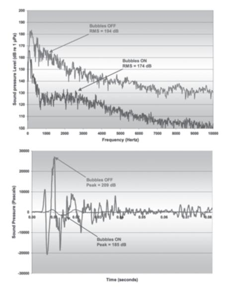
Example waveforms and frequency spectra for 2.4-m-diameter steel pile with and without bubble curtain: Benicia-Martinez Bridge, Carquinez Strait, California. deeper, and the currents stronger. The curtain of air bubbles must be able to extend from the bottom of the pile to the water surface without any gaps.
