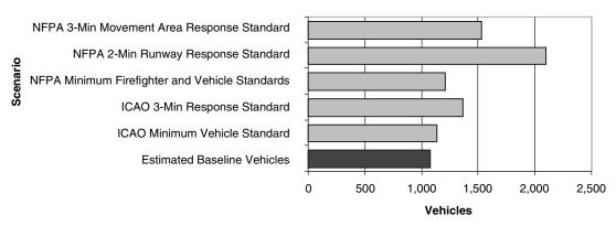
**Figure 8** Summary of baseline firefighters and vehicles required to meet ICAO and NFPA standards at 476 airports.
