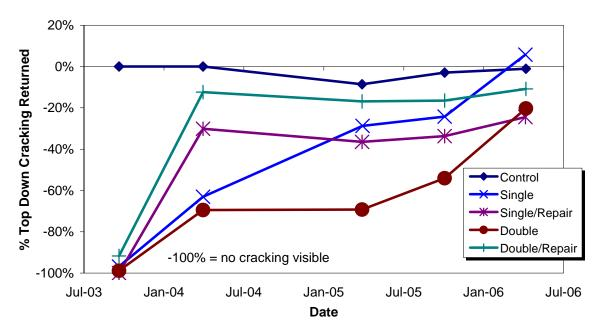
FIGURE 4 Change in reflective (top down) cracking since maintenance activities.
