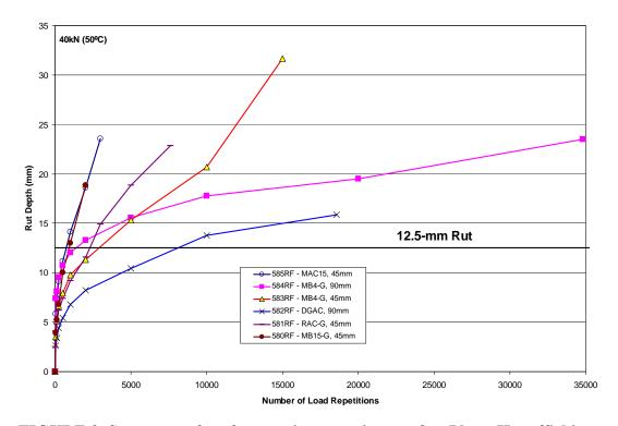
FIGURE 9 Summary of surface rutting experiment after Phase II trafficking.
