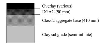
FIGURE 3 Pavement design for test road.
