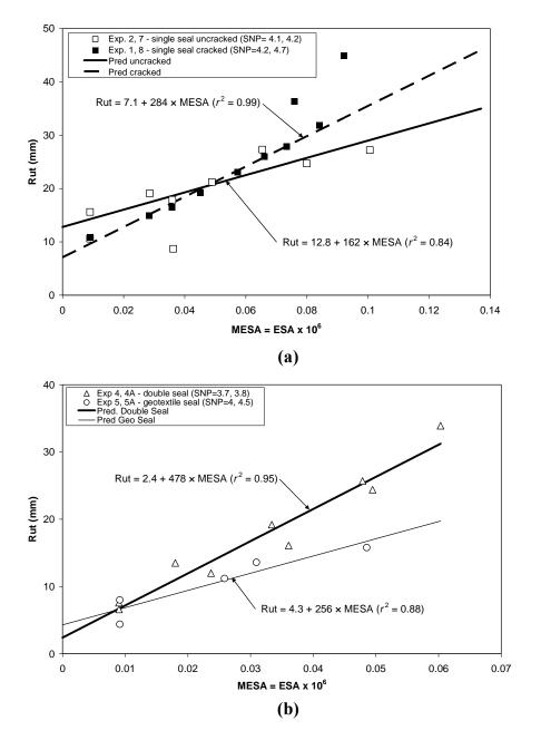
FIGURE 5 (a) Rutting versus loading (MESA) for cracked and uncracked single seals and (b) rutting versus loading (MESA) for double and geotextile seals.
