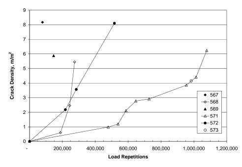
FIGURE 8 Summary of surface cracking after Phase I trafficking.
