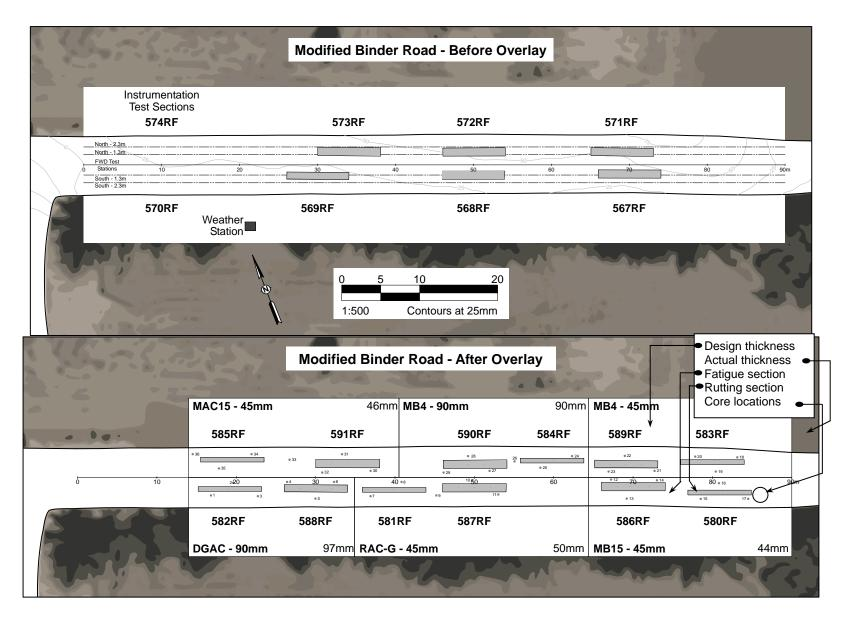
FIGURE 1 Layout of MB road project.
