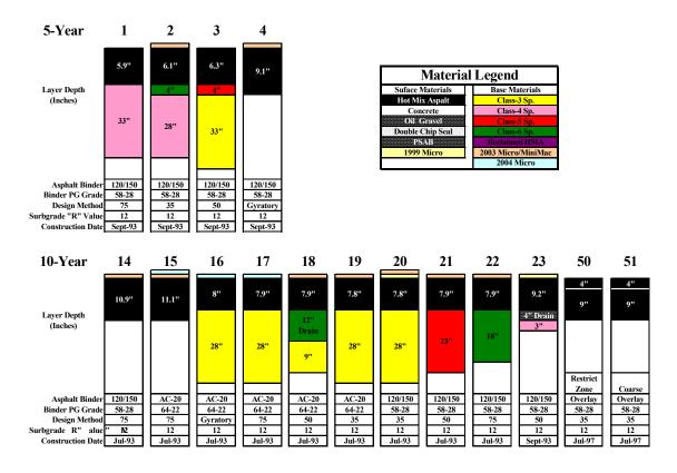
FIGURE 1 MnROAD mainline HMA cell layouts.
