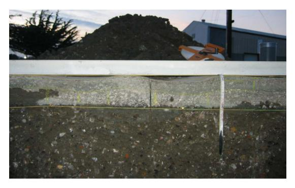
FIGURE 10 Test pit face showing rutting pattern on 45-mm MAC15 and 90-mm DGAC.
