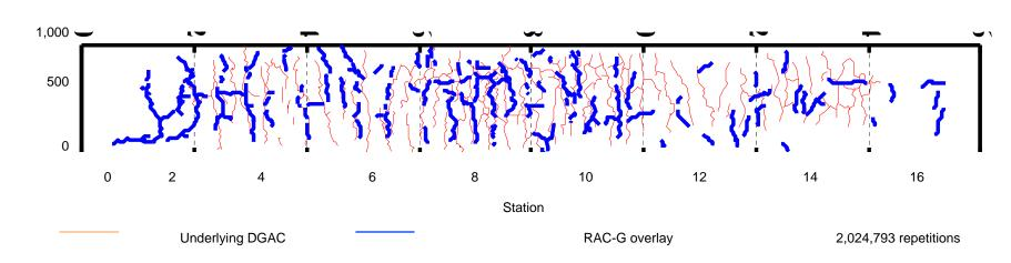
FIGURE 12 Surface cracking after Phase II trafficking showing cracking in both underlying asphalt and overlay.
