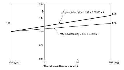
FIGURE 6 Variation in rpf<sub>rut</sub> (*I*/d) and rpf<sub>iri</sub> (*I*/d) with Thornthwaite Moisture Index (uncracked single seals).
