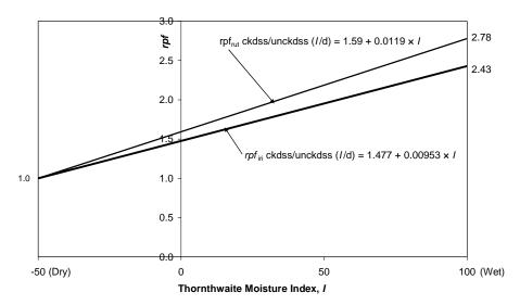
FIGURE 7 Variation in rpf<sub>rut</sub> (*I*/d) and rpf<sub>iri</sub> (*I*/d) with Thornthwaite Moisture Index (cracked single seals relative to uncracked single seals).
