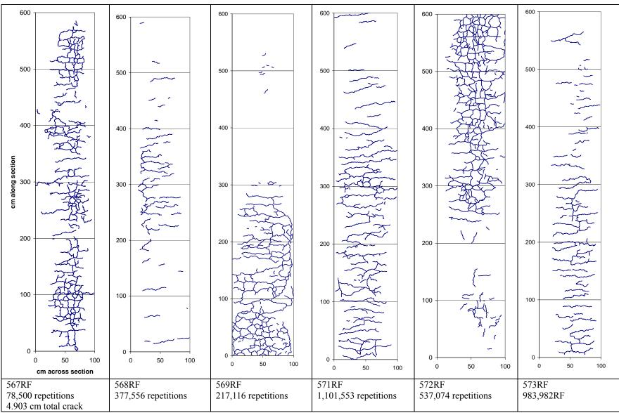
FIGURE 7 Surface cracking after Phase I trafficking.
