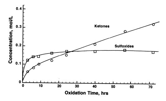
FIGURE 12 Kinetic oxidation data for TFAAT oxidation of SHRP asphalt AAG-1 at 113°C (63).
