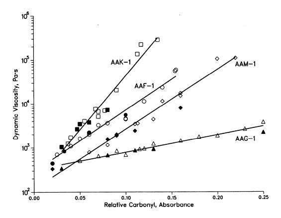
FIGURE 7 Relationships between carbonyls formed and dynamic viscosity increase during PAV (solid points) and TFAAT (open points) oxidative aging (11).
