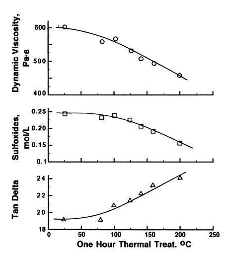
FIGURE 13 Thermal stability of sulfoxides in oxidized SHRP asphalt AAD-1 and effects of their decomposition on rheological properties (91).
