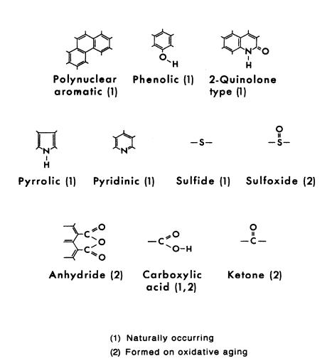
FIGURE 1 Chemical functionalies in asphalt molecules normally present or formed on oxidative aging (1).
