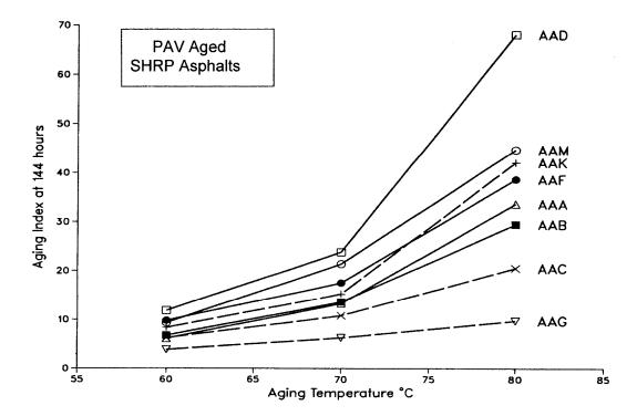
FIGURE 15 Effect of thermal disruption of asphalt microstructure on oxidative age hardening.
