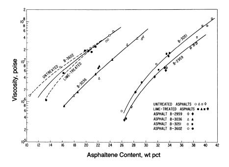
FIGURE 6 Relationship between viscosity at 25°C and asphalene content of untreated and lime-treated asphalts aged by four different laboratory methods (37).
