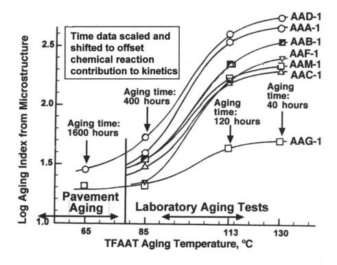
FIGURE 25 Contribution of microstructure to aging index of eight SHRP core asphalts [raw data from Branthaver et al. (63)].
