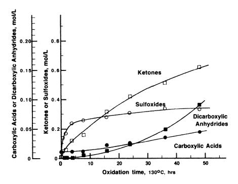
FIGURE 11 Oxidation products formed as a function of time in a Boscan asphalt during thin-film laboratory aging at 130°C (87).
