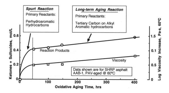
FIGURE 19 Typical kinetics of the dual oxidation mechanism.
