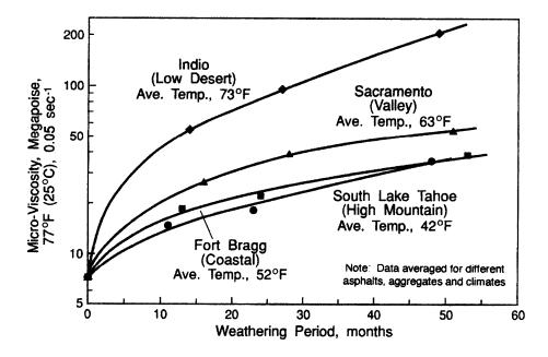
FIGURE 26 Effects of climate temperature on rate of oxidative hardening of pavement mixtures [data adapted from Branthaver et al. (107)].
