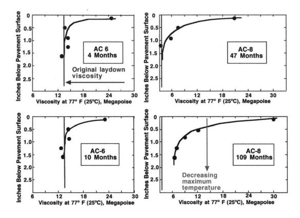
FIGURE 28 Asphalt oxidative age hardening in Georgia pavements as a function of depth. [Plots generated from data in Coons and Wright (111)].
