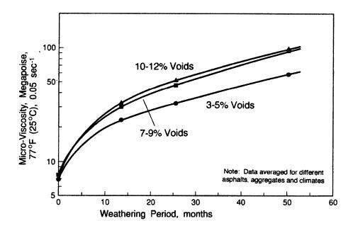
FIGURE 27 Effects of pavement void content on rate of oxidative hardening of pavement mixtures [data adapted from Branthaver et al. (107)].
