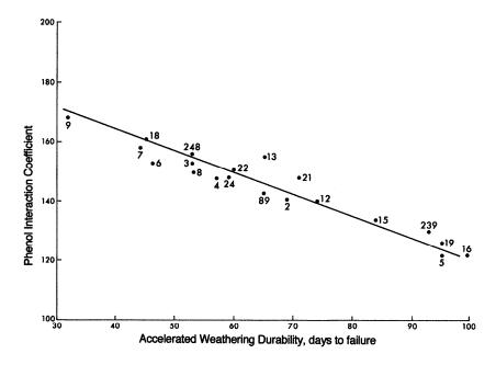
FIGURE 5 Relationship between phenol interaction coefficient and durability of 20 roofing asphalts (66).
