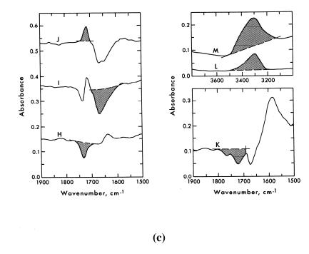
FIGURE 2 (continued) (c) examples of differential infrared spectra used in FGA: H = TPTH treated versus untreated, I = silylated versus untreated, J = silylated versus TPTH treated, K = NaOH treated versus TPTH treated, L = NaOH treated versus solvent, M = untreated versus solvent.
