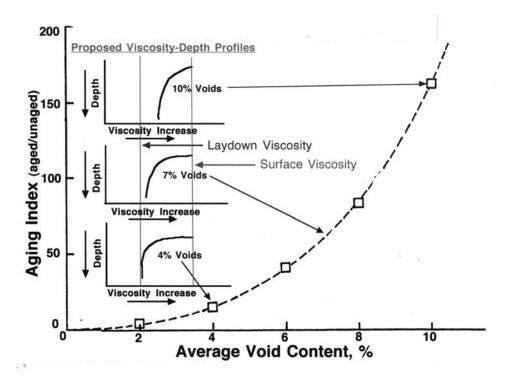
FIGURE 30 Average effect of void content on age hardening of asphalts from 53 11- to 13-year-old pavements. [Graphic produced from Vallerga et al. (112)].
