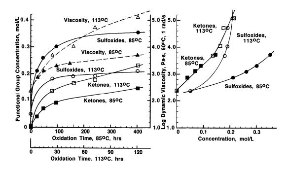
FIGURE 16 Oxidative aging kinetic data and viscosity–functional group relationships for SHRP asphalt AAF-1 after TFAAT oxidation as a thin film at atmospheric pressure (92).
