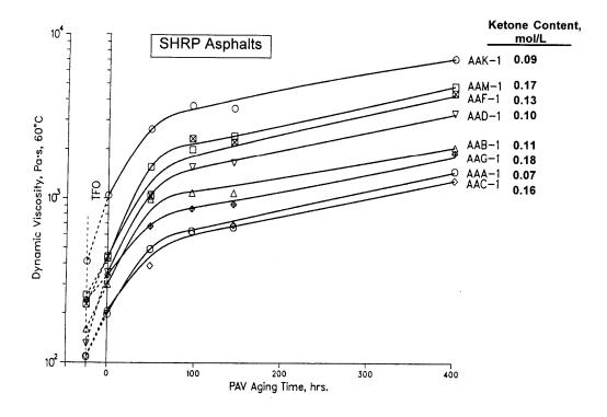
FIGURE 14 Age hardening kinetics of the eight SHRP core study asphalts during PAV in oxygen at 60°C.
