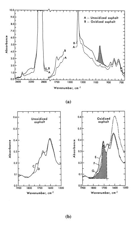
FIGURE 2 (a) Infrared spectra of CS<sub>2</sub> solutions of unoxidized and oxidized asphalt (all spectra solvent compensated) and (b) examples of infrared spectra used in FGA: C = untreated, D = TPTH treated, E = untreated, F = TPTH treated, G = NaOH treated (all spectra solvent compensated).
