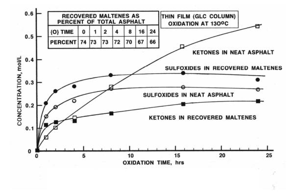
FIGURE 18 Oxidation of a Boscan asphalt: location of the ketones and sulfoxides in the nanodispersion.
