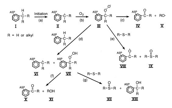
FIGURE 21 Proposed reaction schemes for ketone and sulfoxide formation during oxidation of asphalt benzylic carbon (87, 93).
