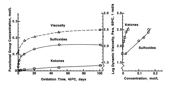
FIGURE 17 Oxidative aging kinetic data and viscosity–functional group relationships for a Shell Wood River asphalt oxidized in air as a thin film on Ottowa sand at 45°C (87).
