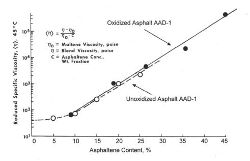
FIGURE 9 Relative size of asphaltene agglomerates in unoxidized and oxidized AAD-1 as a function of asphaltene content as measured by reduced specific viscosity.
