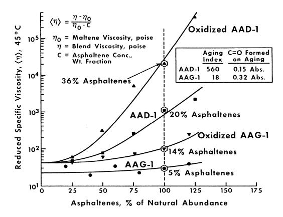
FIGURE 8 Reduced specific viscosity data from measurements at 45°C for asphalts AAD-1 and AAG-1 before and after oxidative TFAAT aging at 113°C for 72 h (11).
