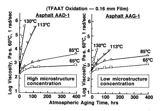
FIGURE 22 Effects of temperature and component compatibility on age hardening kinetics.
