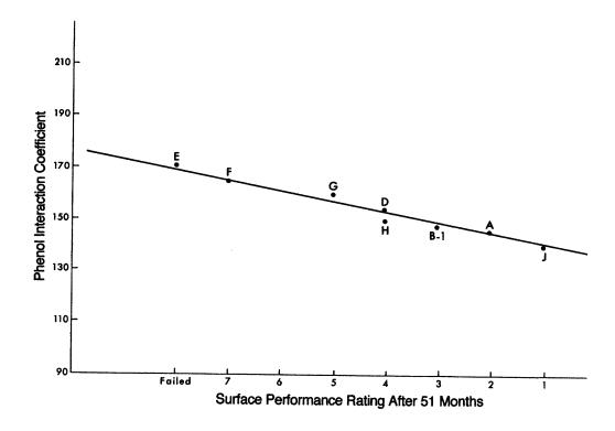
FIGURE 4 Relationship between phenol interation coeffeient and pavement surface performance rating (66).
