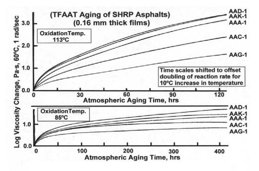
FIGURE 23 Effects of microstructure on age hardening kinetics of five SHRP core asphalts.
