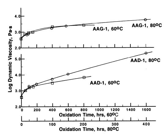
FIGURE 10 Effects of temperature and component compatibility on oxidative aging characteristics (85).
