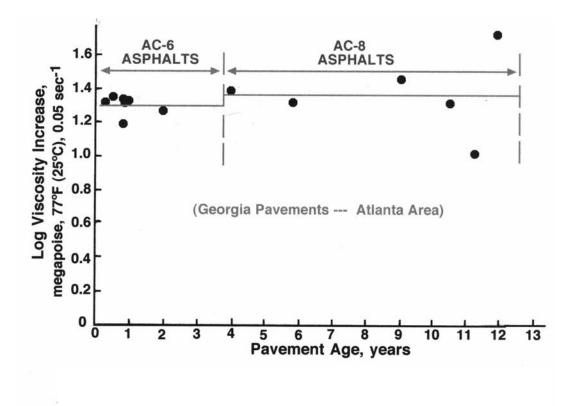
FIGURE 29 Viscosity in the top  $\frac{1}{4}$  in. of pavement in Georgia roads as a function of time in service. [Graphic produced from Coons and Wright (111)].
